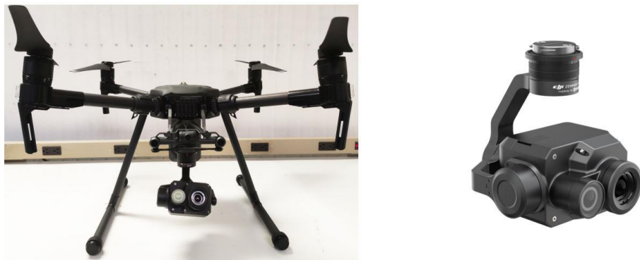
Figure 3.6 DJI MATRICE 200 V2 with ZENMUSE XT 2 imager
