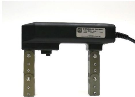
Figure 2.12 Magnetic yoke for magnetic particle testing
