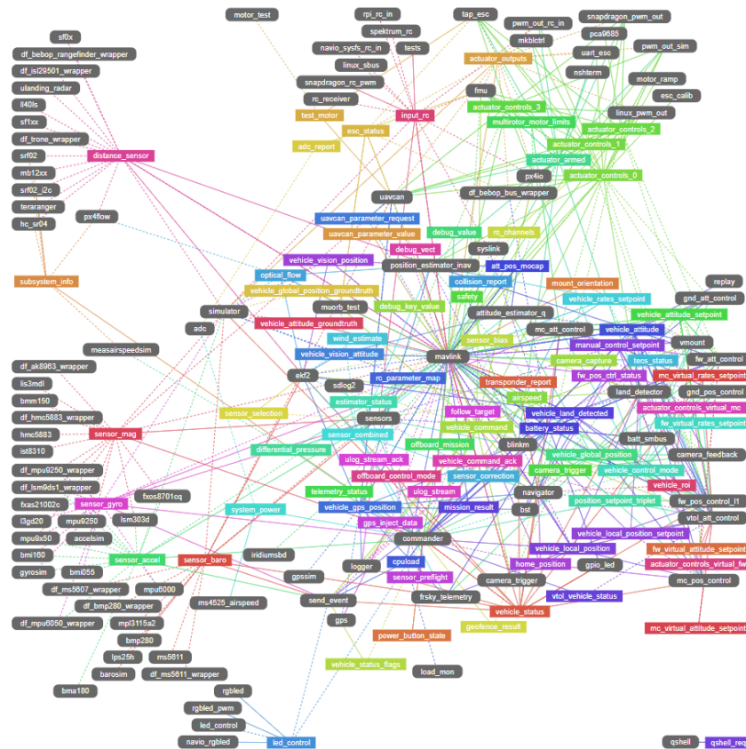
Figure 3.4: uORB schematic. Image source: PX4 developer guide.
