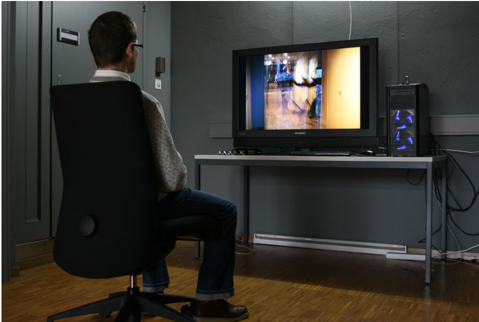
Figure 3.6: . An observer is comparing the original video with an encoded video.[16]
