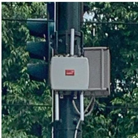
(b) *Meshlium scanner installed on a traffic light pole*
