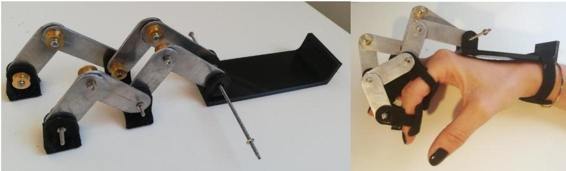
*Figure 26 Exoskeleton structure of the second prototype*
