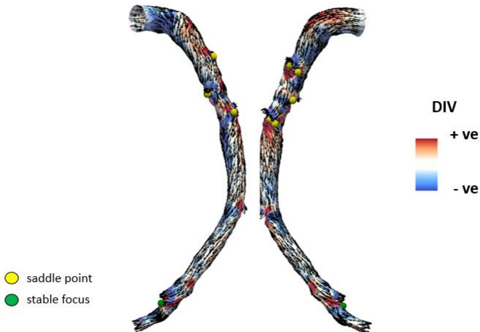
Figure 3.6 WSS topological skeleton of the right coronary artery. WSS manifold are coloured by red (repelling) or blue (attracting). Fixed points were classified as saddle points (yellow) and stable focus (green). Cycle-averaged WSS vector field is displayed by black arrows.
