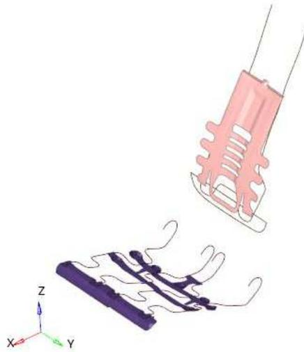
Figure 2.16 Seat spring frames
