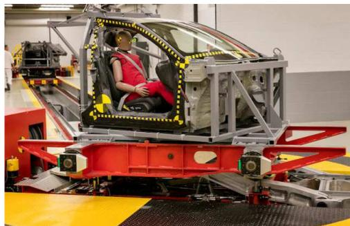
*Figure 2.9 Real sled device*
