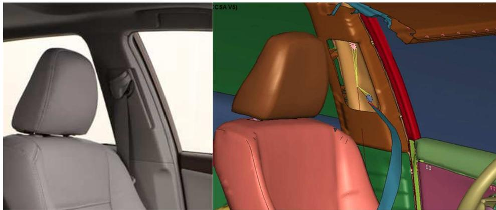
*Figure 2.52 Comparison between actual and FE D-ring position*
