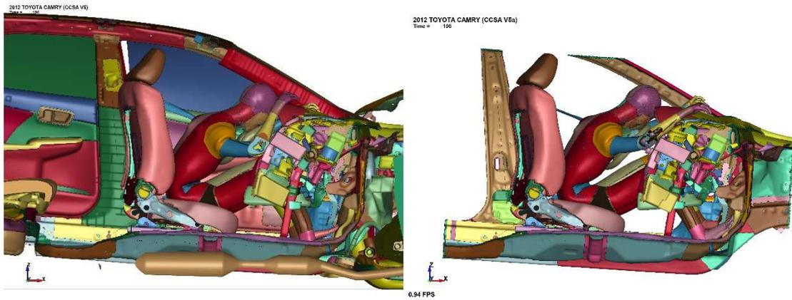
Figure 4.20 Full-scale and sled model with THUMS - side section view - 100 ms
