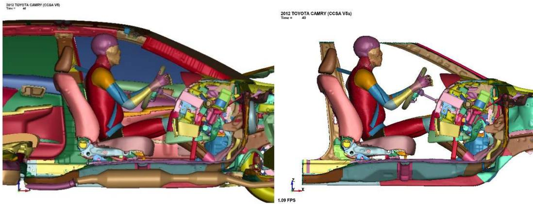
Figure 4.17 Full-scale and sled model with THUMS - side section view - 40 ms
