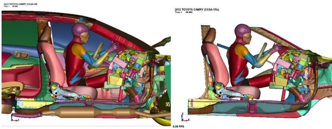
Figure 4.18 Full-scale and sled model with THUMS - side section view - 60 ms
