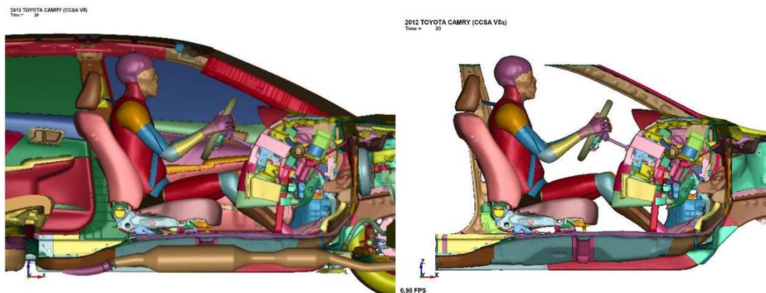
Figure 4.16 Full-scale and sled model with THUMS - side section view - 20 ms
