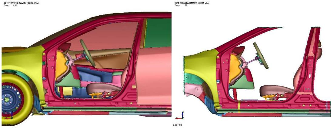
Figure 4.2 Full-scale and sled model - side view - 20 ms
