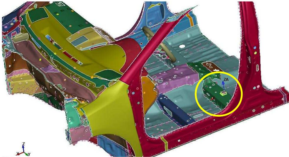
Figure 2.38 Sled model - Driver accelerometer
