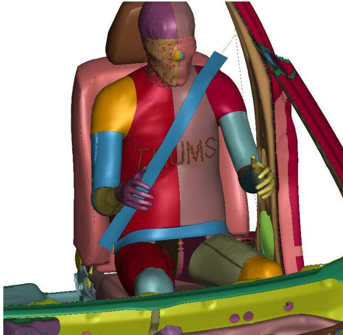
*Figure 3.19 Seatbelt model at the end of the routing*
