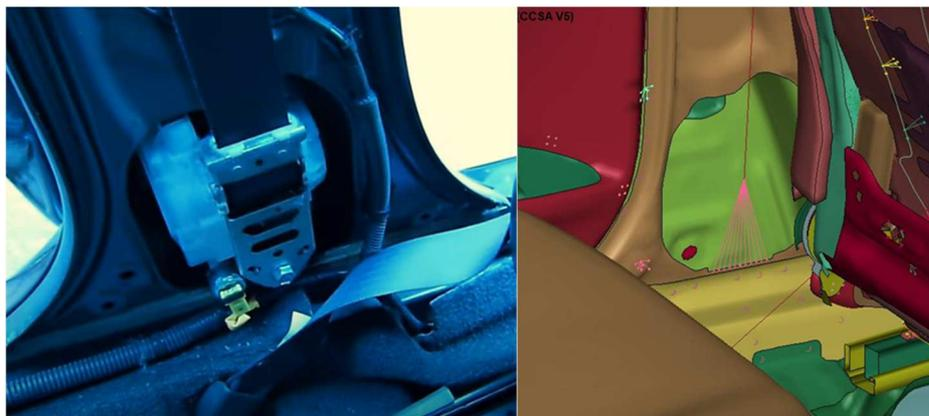
*Figure 2.53 Comparison between actual and FE retractor position*
