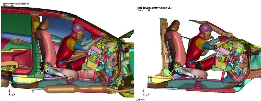
Figure 4.19 Full-scale and sled model with THUMS - side section view - 80 ms
