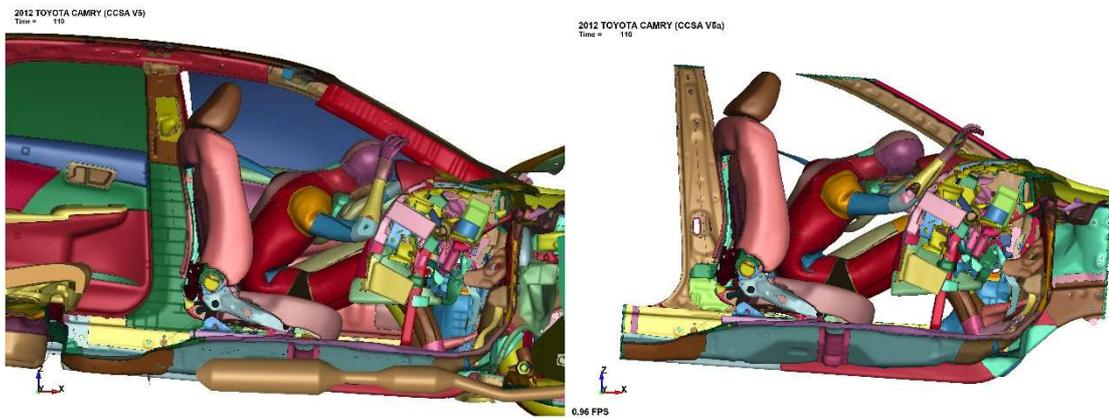
Figure 4.21 Full-scale and sled model with THUMS - side section view - 110 ms
