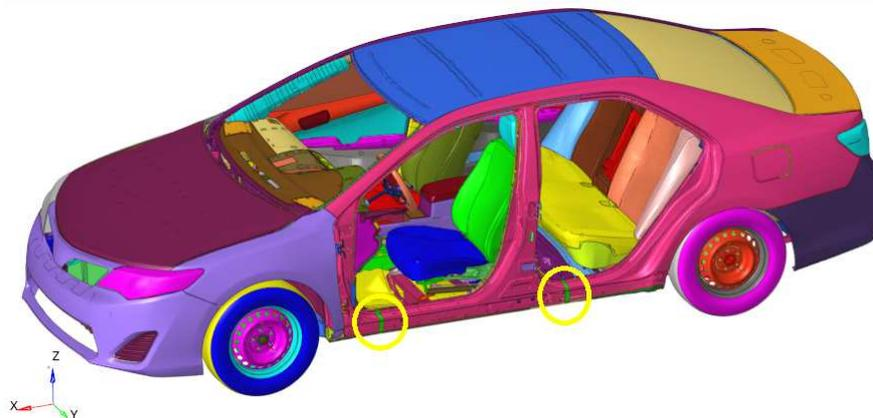
Figure 2.25 Detail of rigid sections position in Rigidparts model
