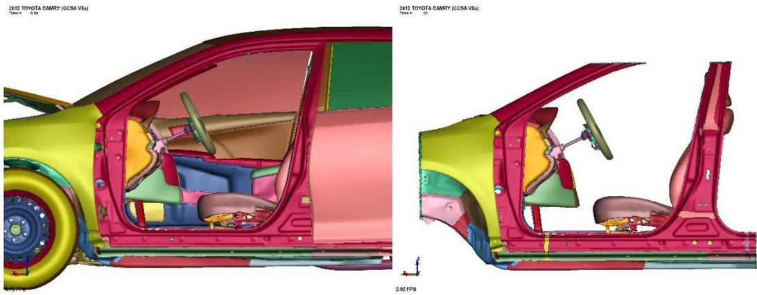
Figure 4.3 Full-scale and sled model - side view - 40 ms
