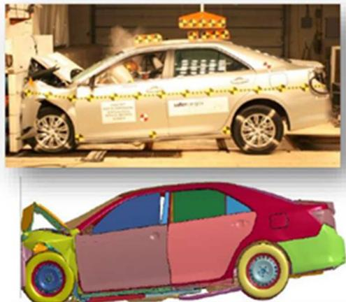
*Figure 2.1 Real NCAP crash test and NCAP simulation*
