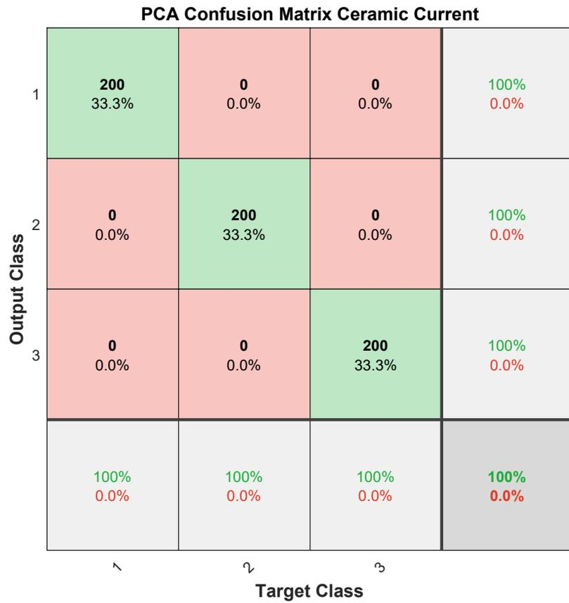
Figure 6.25: Confusion Matrix PCA, for stator current measurements of ceramic bearings
