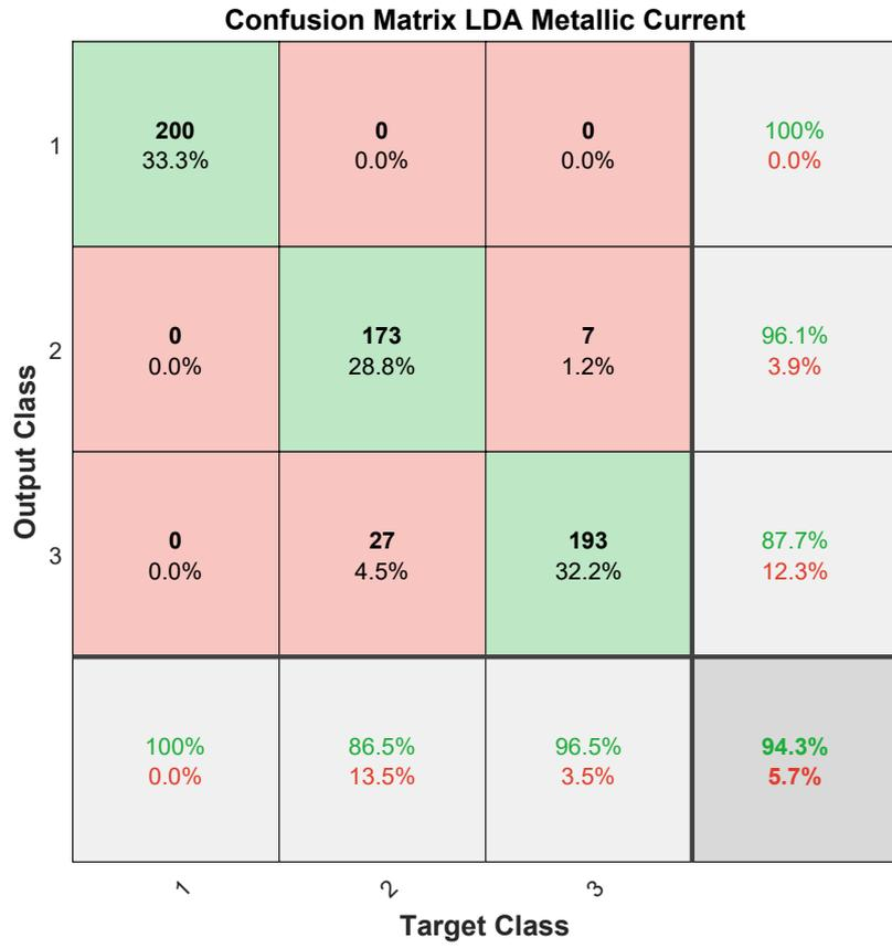
Figure 6.27: Confusion Matrix LDA, for stator current measurements of metallic bearings
