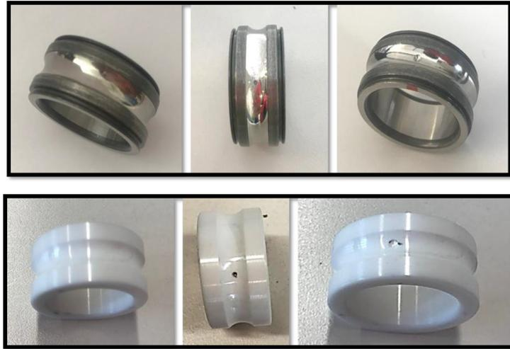
Figure 4.2: Metallic and ceramic bearing mounted on the shaft
