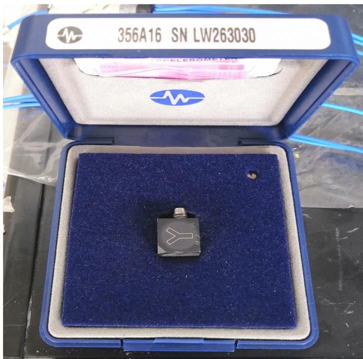
Figura 4.2: Accelerometro *Piezotronics* [15]
