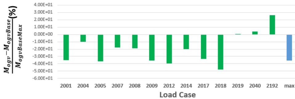
Figure 6.7: OGV bending moment variation compared to baseline for  $FRMX$  configuration
