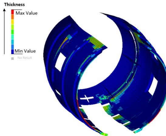
Figure 4.3: Thickness distribution as result of the FS optimization for the C-duct configuration
