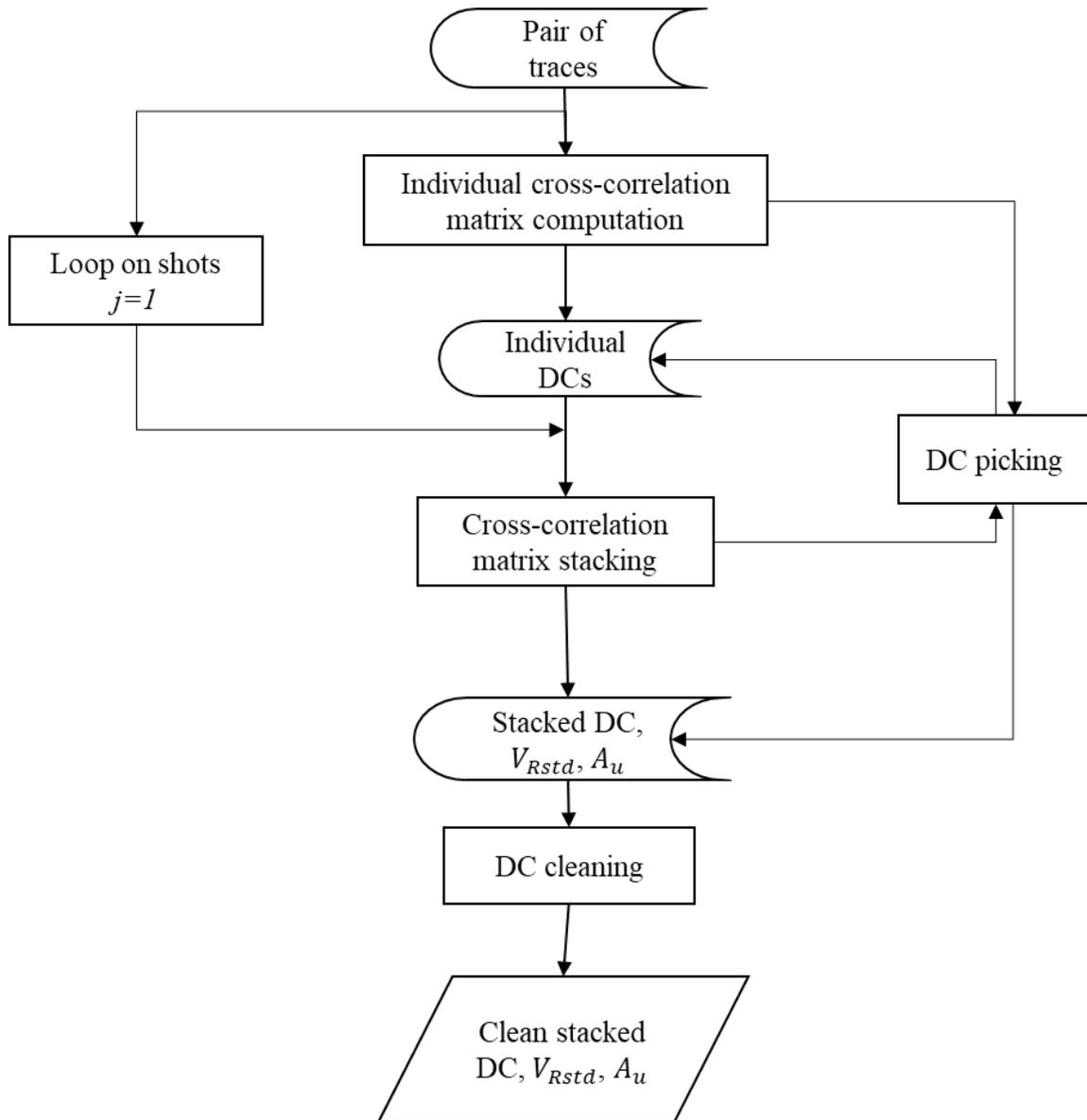
Figure 3.3. Workflow of the automatic DC picking method (Papadopoulou, personal communication)
