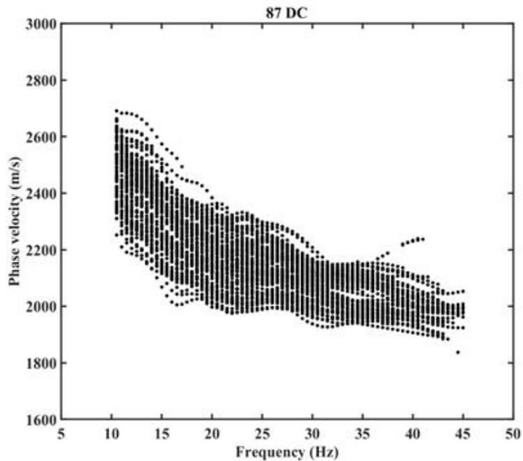
Figure 4.2. DCs relevant to those 87 receiver pairs from which the manually picked DCs have been saved. Line 1.
