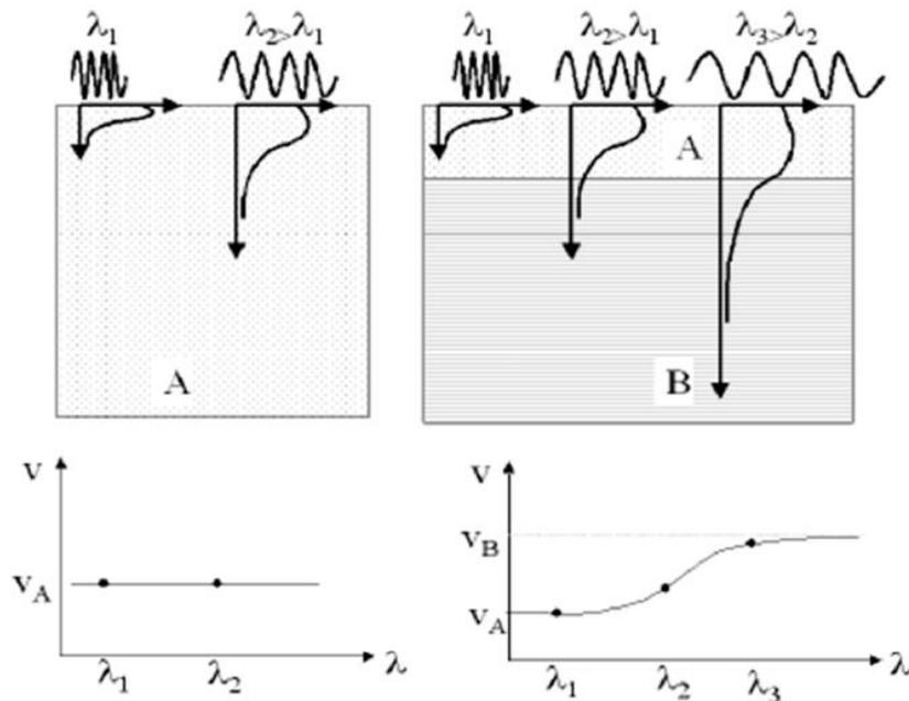
Figure 1. 2. Difference in velocities in various environments. a) Homogeneous environment; b) Heterogeneous environment, where the velocity of wave propagation depends on the wavelength (Strobbia 2003).
