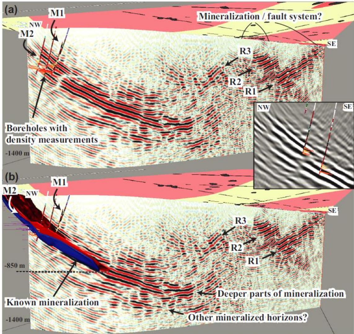
Figure 2. 2.A 3D visualisation of the seismic section with a) boreholes with density measurements on the right-side closer, b) blue and red surfaces that represent 850m of the known portions of the mineralisation and possible extension of it down to 1200 m (Markovic ad et.2019)
