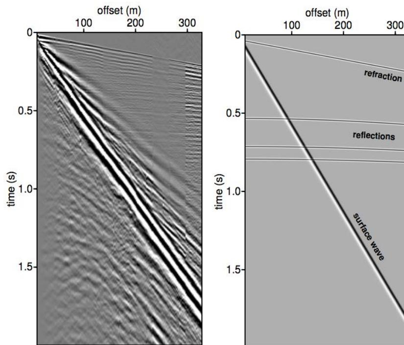
*Figure 1. 1. Seismic events obtained from the seismic survey (Drijroningen, 2011).*
