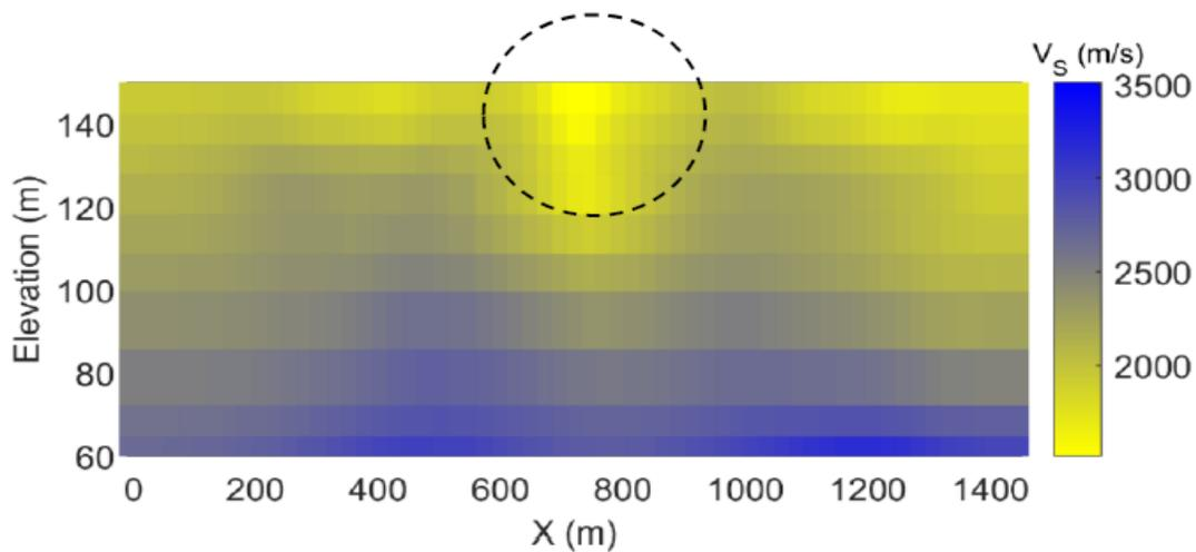
Figure 2. 3. Figure 2.3. Result of the inversion. The strong anomaly caused by a local discontinuity is highlighted with a dashed circle (Papadopoulou et al. 2019).
