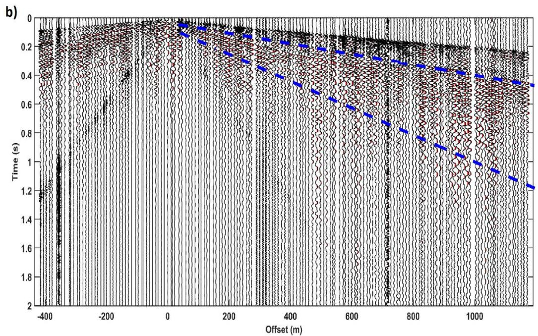
Figure 2. 7. Examples of seismic records obtained from the field. Dashed blue lines highlight SWs.
