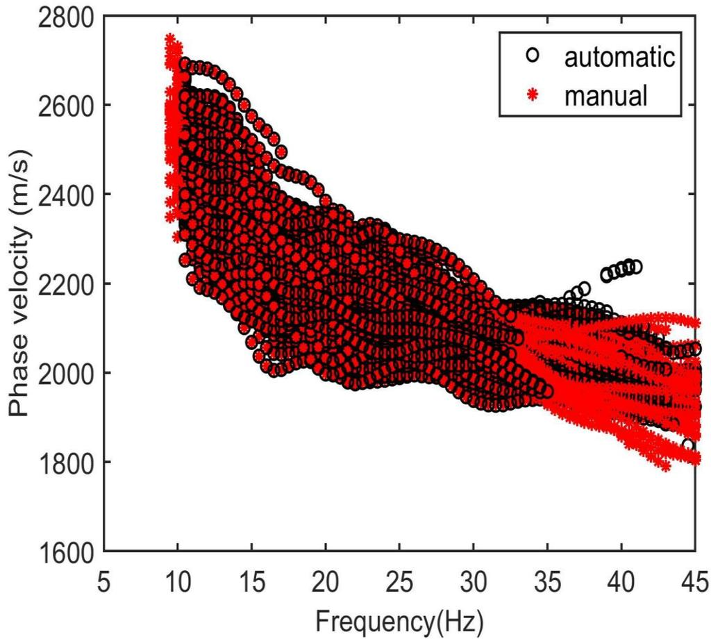
Figure 4.3. *Superposition of 87 DCs retrieved by manual and autopickings. Where the red colour characterises manually picked DCs, while black ones.*
