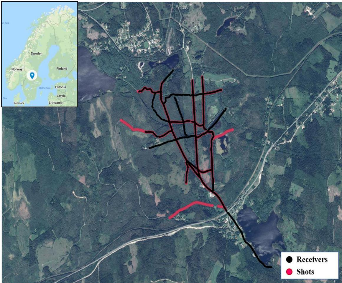
*Figure 2. 5. Seismic Acquisition scheme of Ludvika mining area of Blötberget, Sweden. Acquisition date: April 27 – May 18, 2019. Black dots represent receivers, while red dots stand for shots.*
