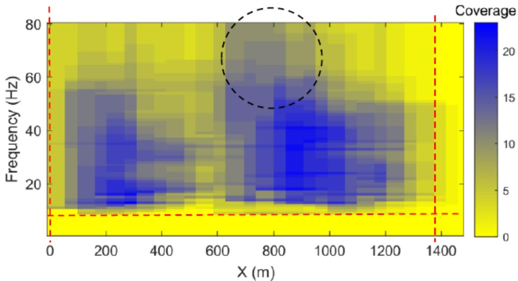
Figure 2. 4. Coverage of the data along the line. Dashed lines indicate the range of the frequencies and positions that provided coverage >0, which also includes the anomaly zone (dashed circle). (Papadopoulou et al. 2019).
