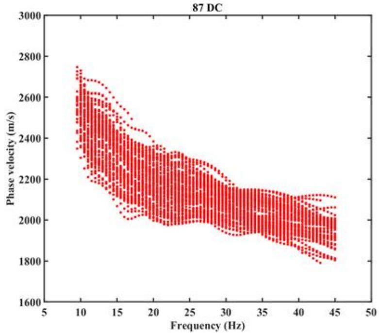
Figure 4.1. Manually picked DCs from 100 receiver pairs' seismic data relevant to Line 1.
