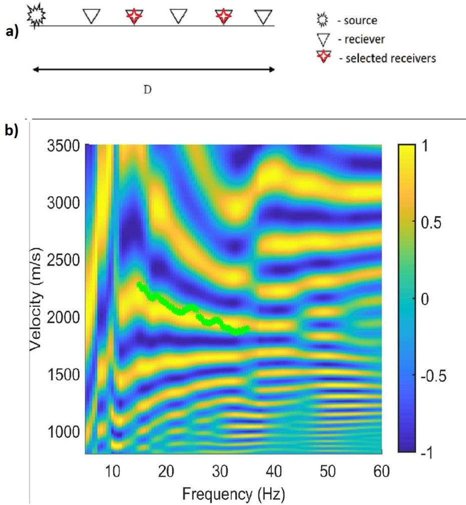
Figure 1. 4. (a) An example of the selection of a pair of receivers, which are indicated with red stars, for the two-station method; (b) a cross-multiplication matrix, represented in phase velocity and frequency domains, the green stars represent reference curve.
