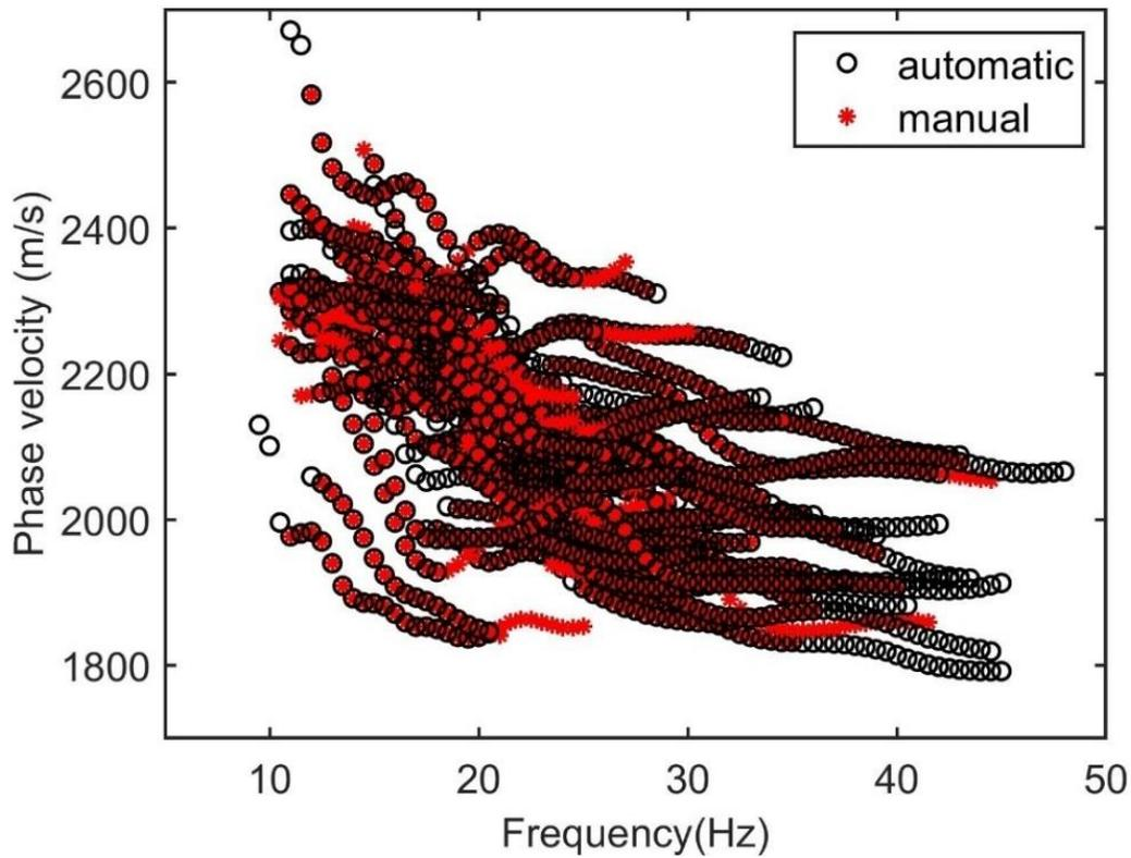
*Figure 4. 4. Superposition of 65 DCs retrieved by manual and automatic DC pickings from the seismic data of 200 receiver pairs allocated on Line 2.*
