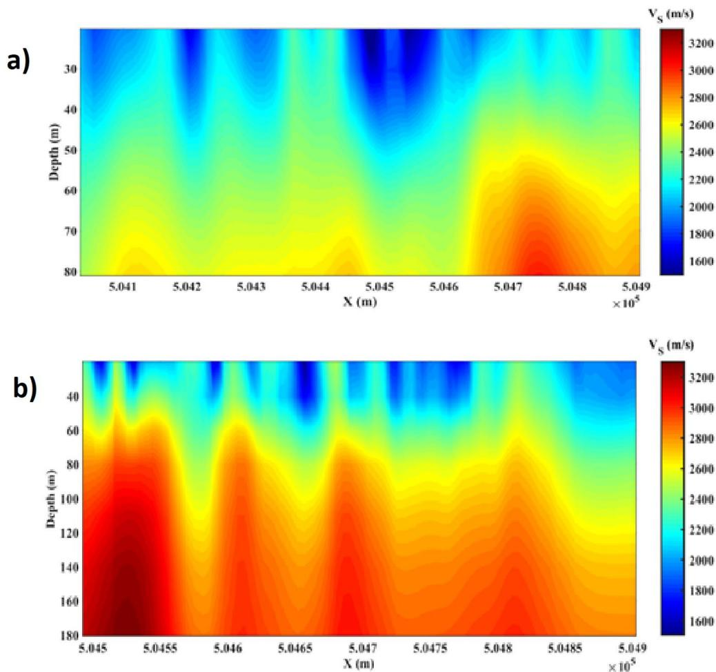
Figure 4. 13. Shear wave velocity profiles retrieved from the inversion of DCs of a) Line 1 and b) Line2 (Papadopoulou, personal communication).
