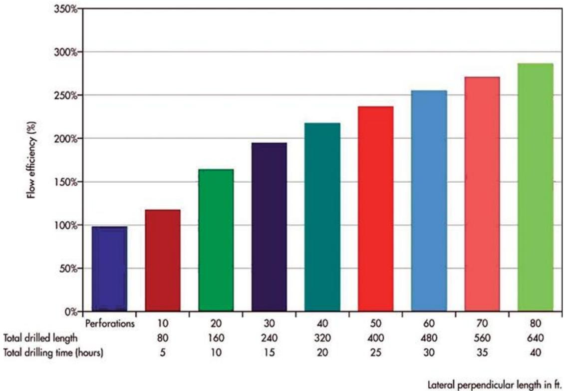
Fig. 4.24: Comparison of perforation Flow efficiency versus laser drilled laterals
