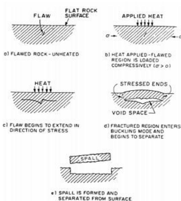
Fig. 4.5: Thermal Spallation
