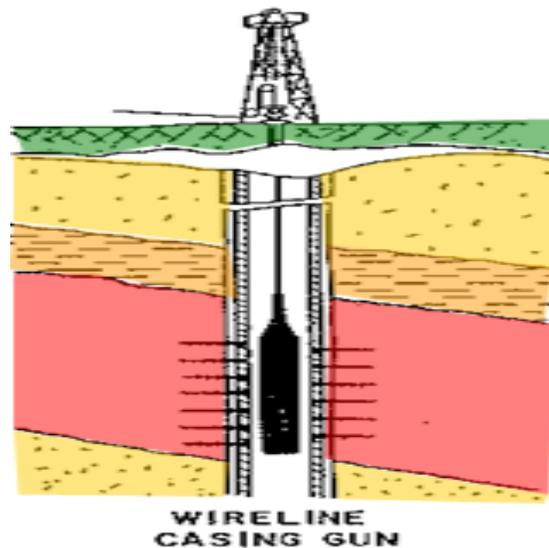
Fig. 2.7: wireline casing gun
