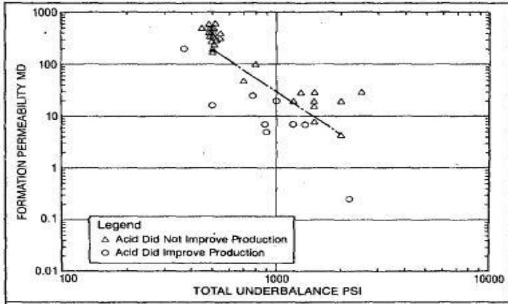
Fig. 2.13: Underbalance used on TCP in sandstone oil zones (King et al., 1986)
