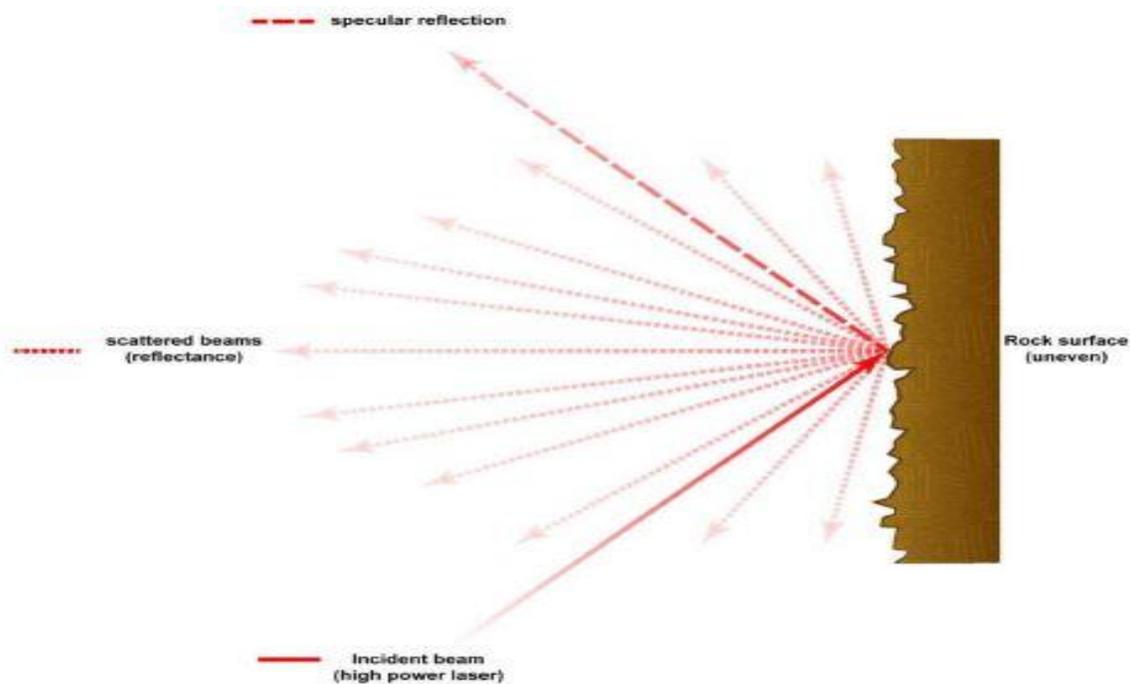
Fig. 4.3: Oblique incidence of reflection and scattering
