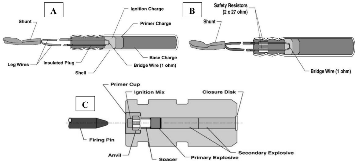
Fig. 2.4: Detonator types
