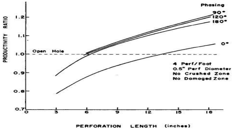
Fig. 2.17: phasing effect on productivity ratio (Locke, 1981)
