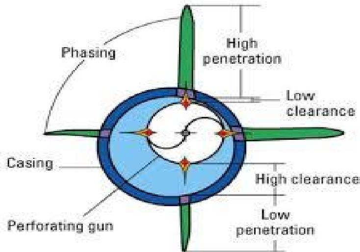
Fig. 3.3 Perforation penetration (taken from Schlumberger Oilfield Glossary, 2020)
