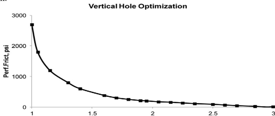
Fig. 4.8: Friction pressure of perforation as a function of perforation diameter
