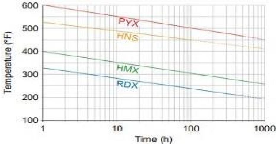
Fig. 2.6: stability temperature for perforating explosives
