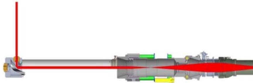
Fig. 4.21 Showing Angle beam orientation mode in Laser perforation gun
