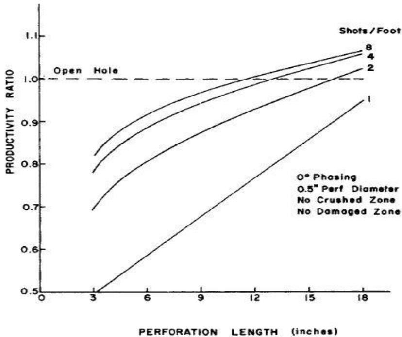
Fig. 2.14: Productivity ratio versus perforation length (Locke, 1981)
