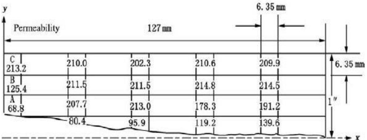
Fig. 3.7: Distribution of permeability ( $10^{-3}\mu\text{m}^2$ ) around perforation (Asadi & Preston, 1994)
