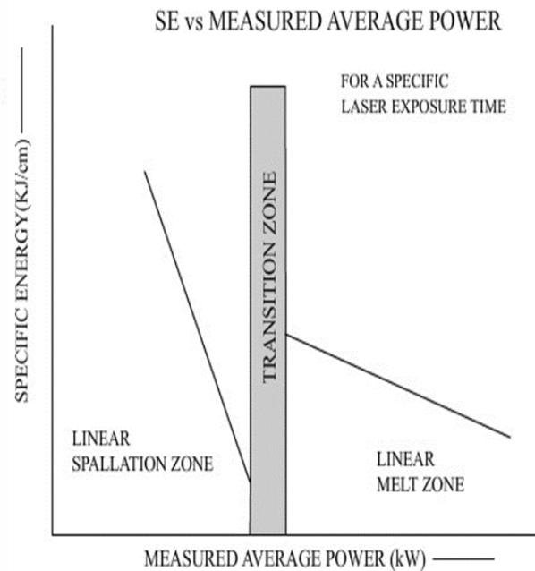
Fig. 4.6: Spallation and melting Zone
