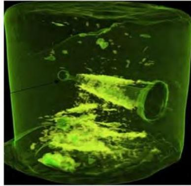
Fig. 4.11: CT-scan in unconsolidated sand laser perforation
