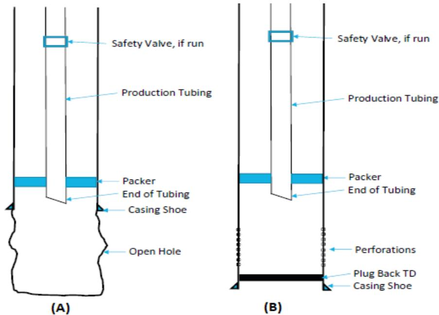
Fig. 1.1 Open hole and cased hole completion
