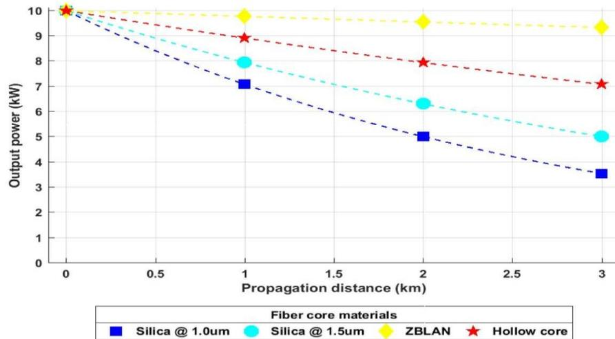
Fig. 4.16: 10kW laser beam optical loss of different fiber types as a function of distance(Batarseh et al., 2019b)
