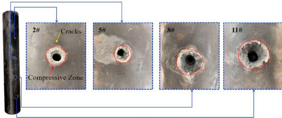
Fig. 3.4 Characteristics of the cement surface damage after perforation.
