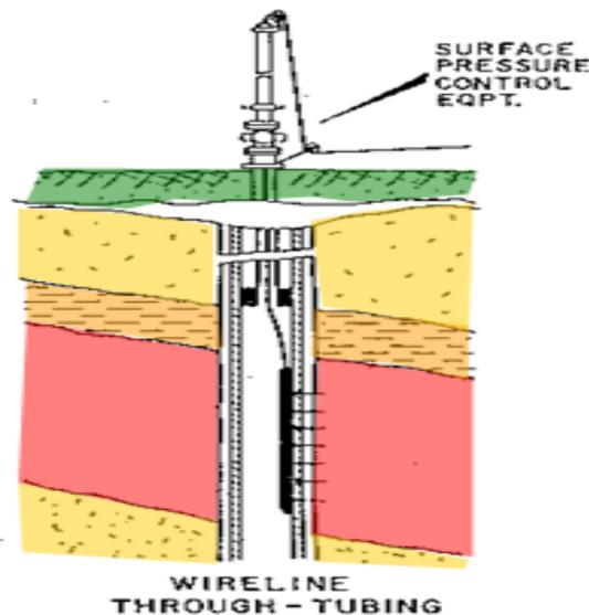
Fig. 2.8 Through tubing gun
