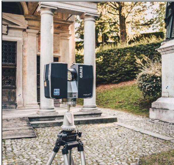
Figura 54 - Laser scanner FARO CAM 2.
