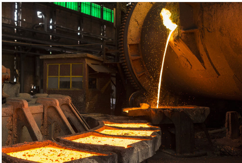
Figure 1.9. Liquid material poured into rotating moulds, from Encycl. B. (2020) .
