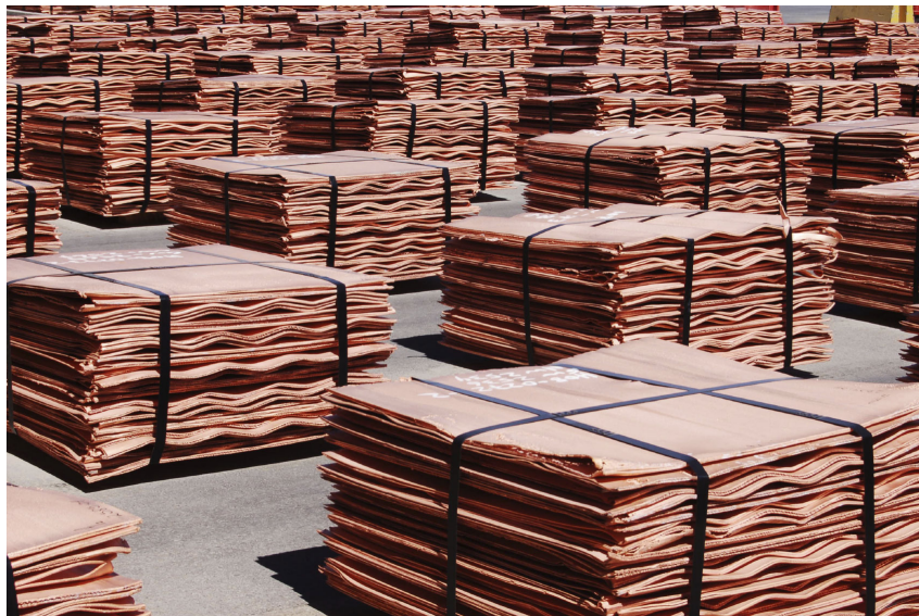
Figure 1.12. Storage plant of copper cathodes with minimum 99.99% of copper content, ready for worldwide shipping. Photo retrieved from www.reinhausen.com .
