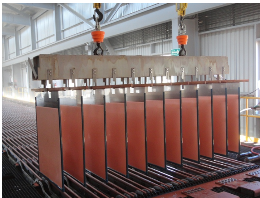
Figure 1.10. Copper electrorefining tankhouse, from Copper Alliance (2020) .
