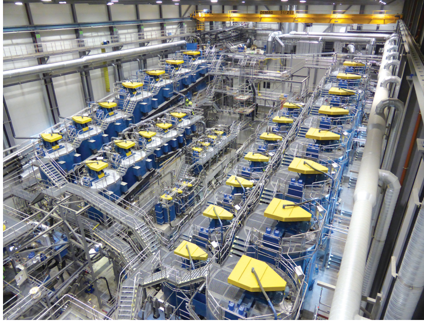
Figure 1.8. Series of tanks used in copper Froth Flotation plant, from Leonida (2020) .
