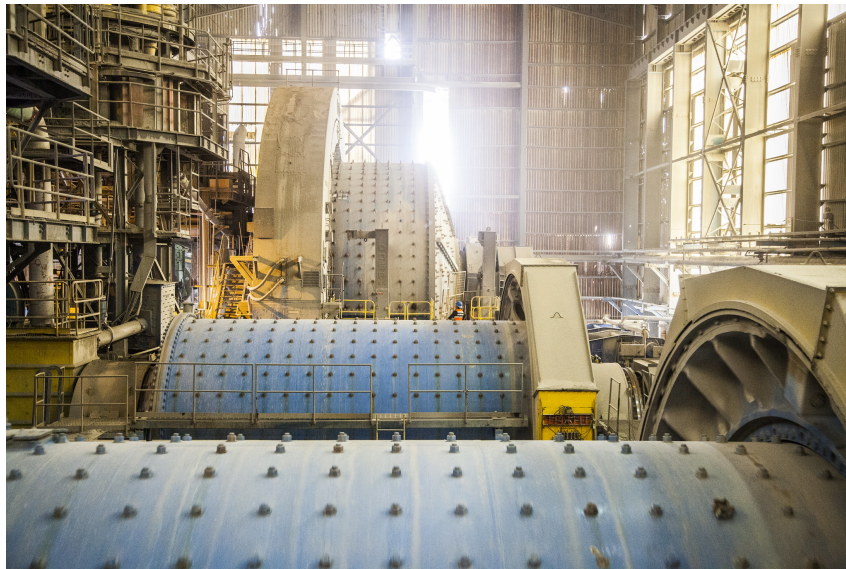
Figure 1.7. Primary comminution in El Teniente mine, from Gleeson (2020).
