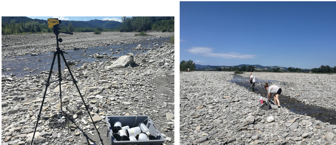
FIGURE 2.9: TruPulse laser rangefinder 360B telemeter used during the biological surveys (on the left) and measuring of velocity and depth in a sample point with Marsh-McBirney Flow-Mate current meter (on the right)
