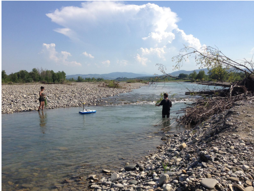
FIGURE 2.4: ADCP on the floating platform acquiring depth and velocity data.
