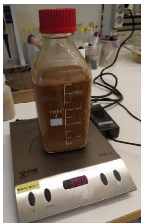
Figure 4.2 Stirring of lignin with ethylacetate during the fractionation step
