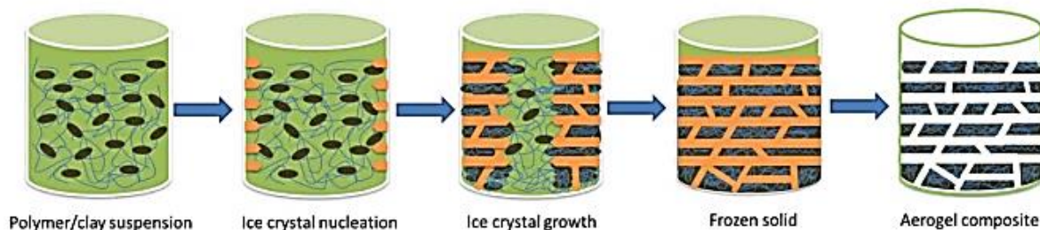
Figure 5.4 Schematic representation of the scaffold production process[89]
