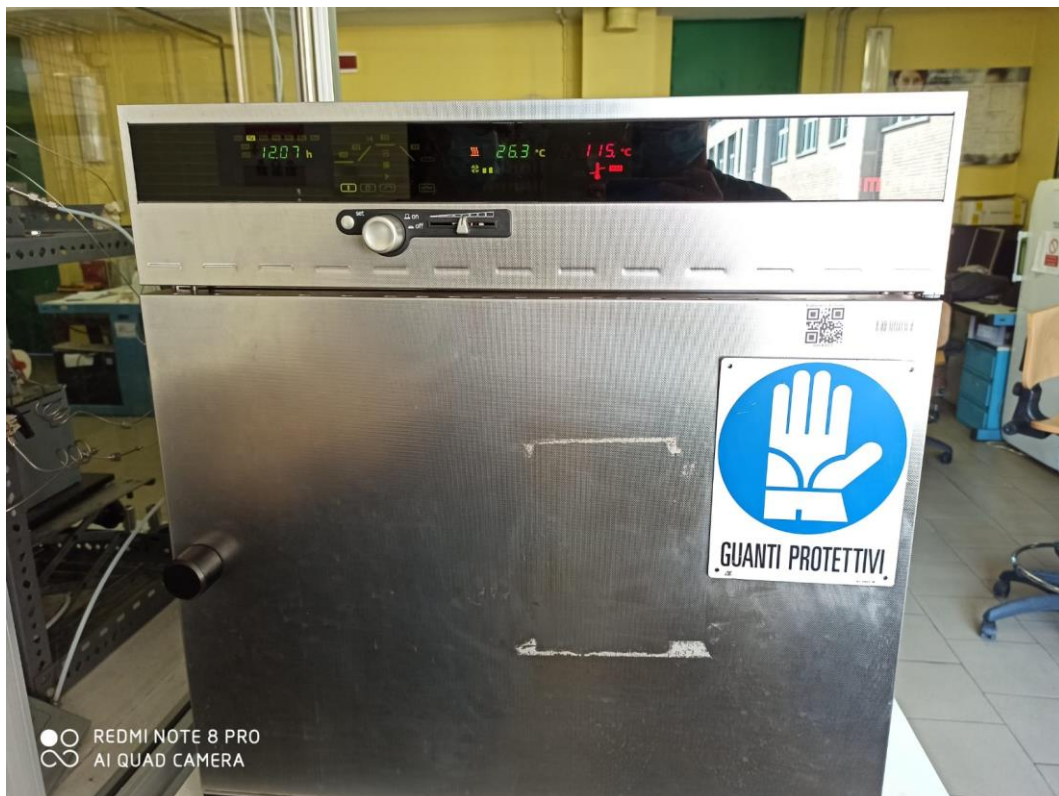
Figure 2.1 - Picture of the oven used in the DISAT laboratory to perform the moisture content analysis. (Picture of Giuseppe Pipitone)
