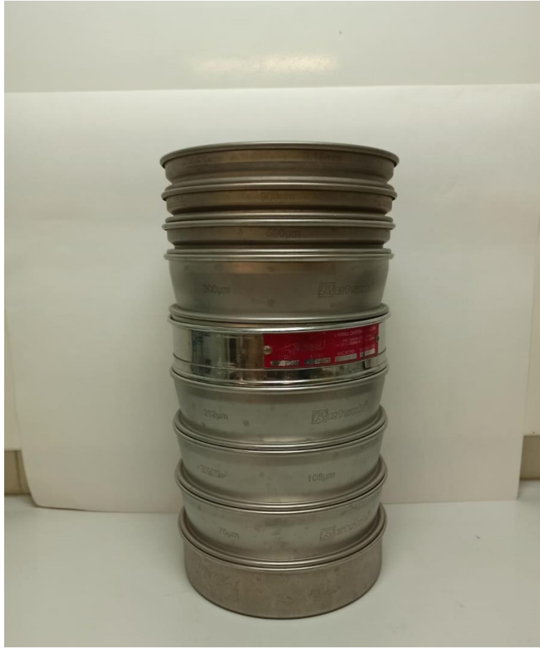
Figure 2.6 - Picture of the sieves columns used to perform the sieve analysis. (Picture taken by Giuseppe Pipitone)
