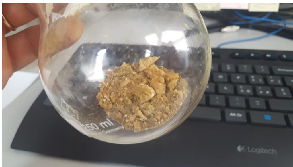
Figure 2.9 - Dry solid extract (after freeze drying). Picture taken by Giuliano Cavaglià.
