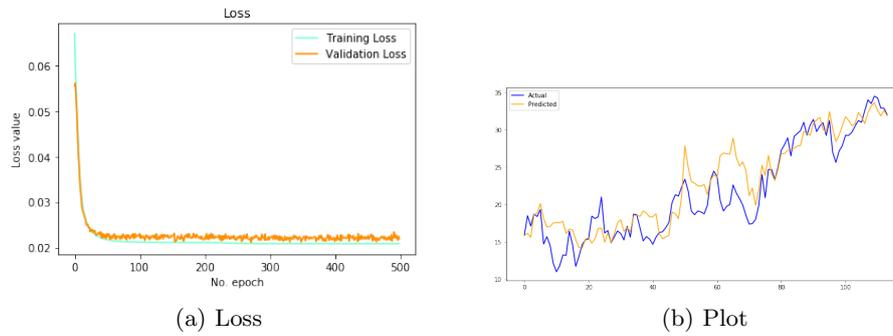
Figure 4.13: Figure on the left shows both training and validation loss for the classical FFNN. In the picture on the right we see real and predicted values on test set.
