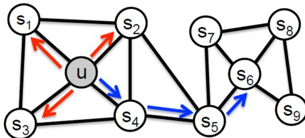
Figure 3.1: Generation of a neighborhood set of given cardinality equals to 3 for node  $u$ , according to the two different sampling strategies. In red the BFS-neighborhood  $(s_1, s_2, s_3)$ . In blue the DFS-neighborhood  $(s_4, s_5, s_6)$ . Figure from [9]
