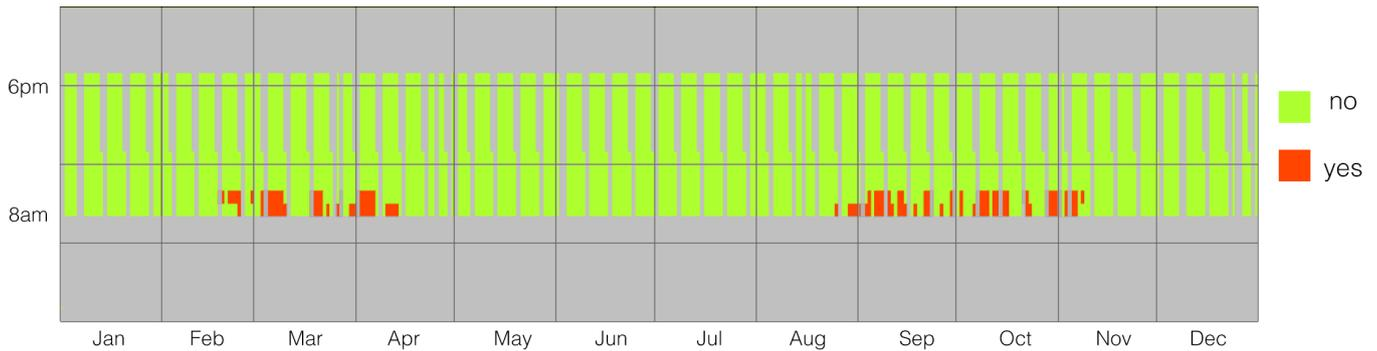
Figure e4.36 Annual glare simulation - point 71 (see figure a.22 pag 59)
