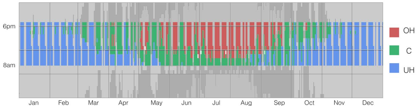
Figure b2.4 Mean Overheated, Comfort and Under-heated annual plot ranges - free running simulation
