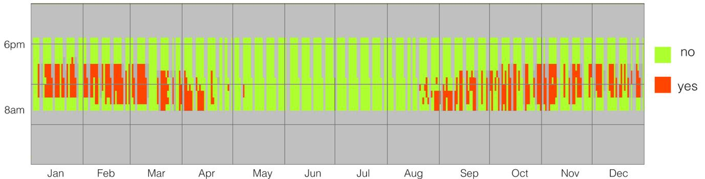
Figure c3.32 Annual glare simulation - point 58 (see figure a.22 pag 59)
