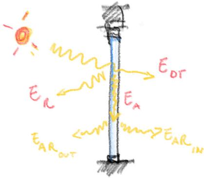
Figure c1.1 Concept scheme of solar energy through glazing
