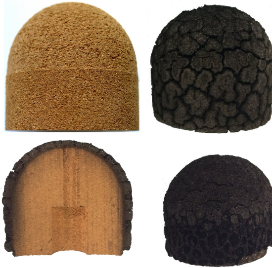
Figure 2.3: On the top: surface of the cork P50 from virgin (left) to fully charred (right), after a test in Plasmatron. On the bottom: section of the charred sample. Pictures taken from [7].
