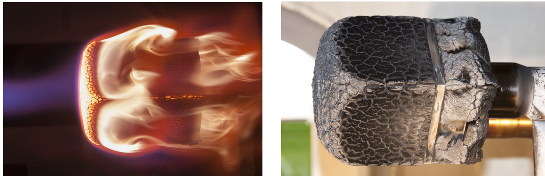
Figure 1.12: QARMAN sample during (left) and after (right) the test in Plasmatron. Figure modified from [7].
