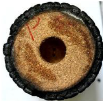
Figure 2.4: Back view of fully charred cork P50, after a test in Plasmatron. Picture taken from [50].
