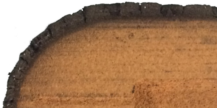
(c) Section of a P50 sample after a test in Plasmatron conducted by Sakraker [7].
