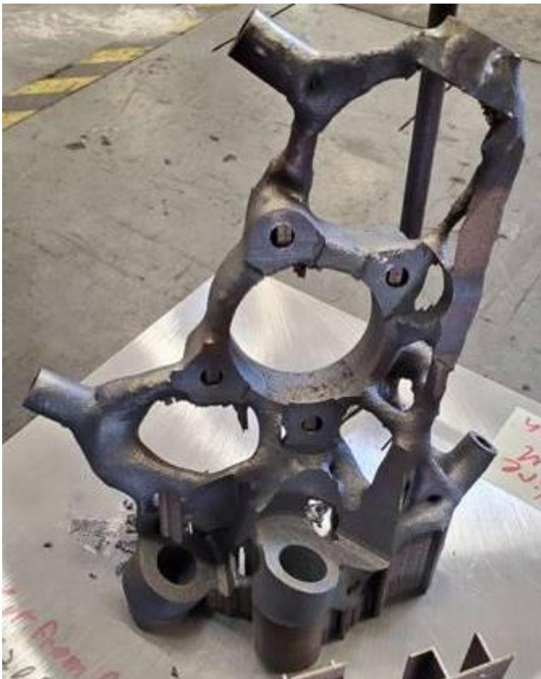
*Figure 6-53 Support removal process on the optimized component*
