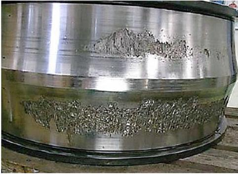
(a) Spalling fatigue failure
