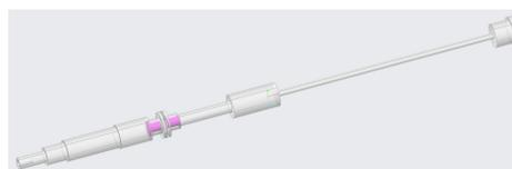
Figure 4.39: Shafts assembly bounded contact
