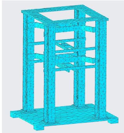
Figure 4.18: Medium mesh, complete external structure
