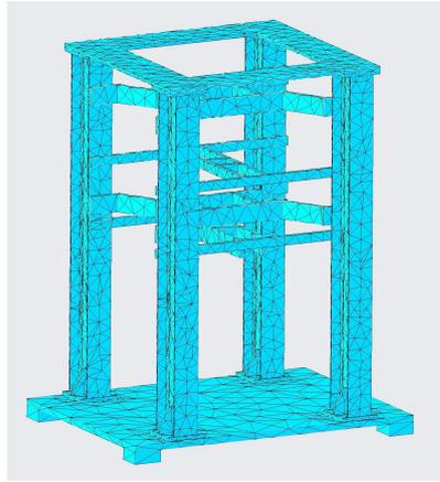
Figure 4.17: Coarse mesh, complete external structure
