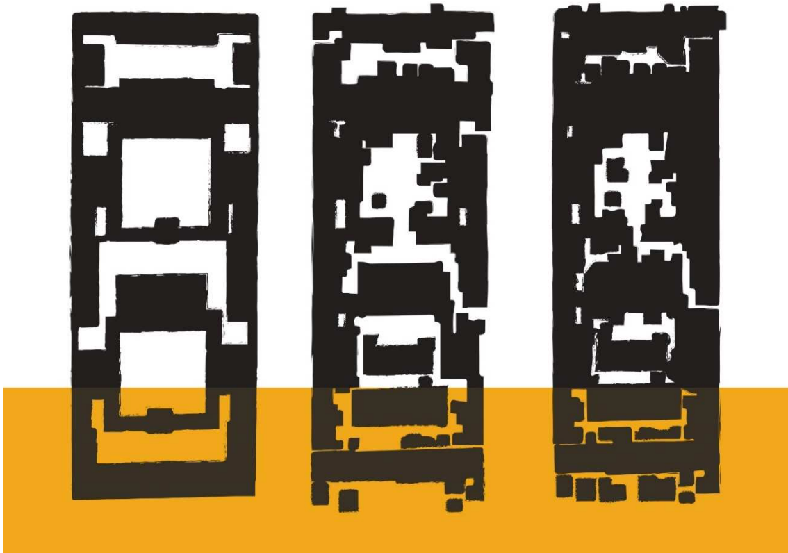
Figure 4.17 Densification of the hutongs , a) 1950s, area of 2441 sqm b) 1970s, area of 3197 sqm c) 1987, area of 3787 sqm (Y. Wang 2016)
