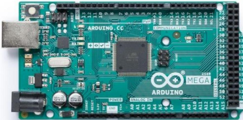
Figura 2-11: Arduino Mega 2560
