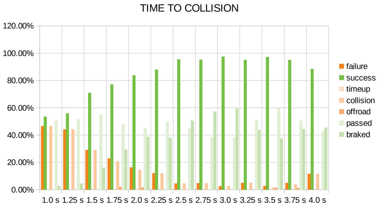
Figure 5.7 Results of Autonomous Emergency Braking Test – Time To Collision
