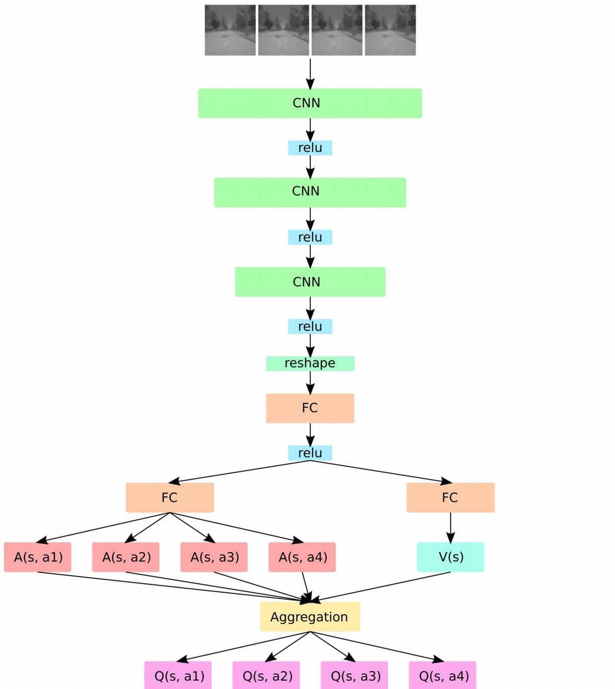
Figure 4.9 Autonomous Emergency Steering Neural Network
