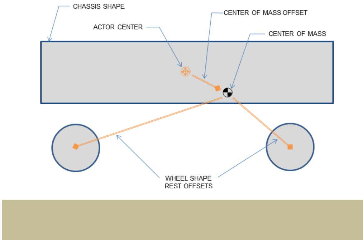
Figure 3.3 Vehicle representation as a rigid body actor [33]
