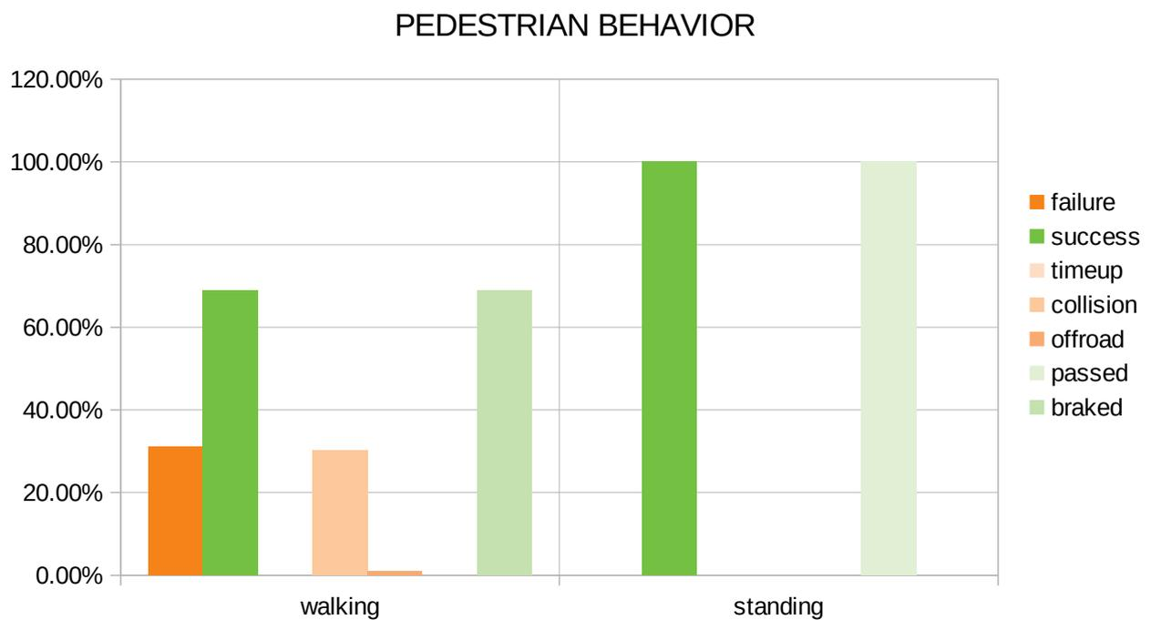
Figure 5.5 Results of Autonomous Emergency Braking Test – Pedestrian Behavior
