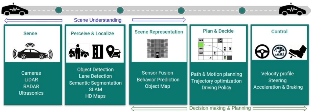
Figure 3.1 A modern Autonomous Driving System pipeline [23]
