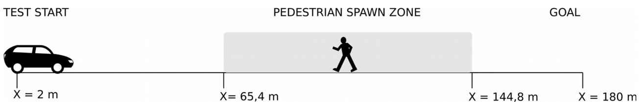
*Figure 4.8 Autonomous Emergency Steering test Spawning and Goal Positions*
