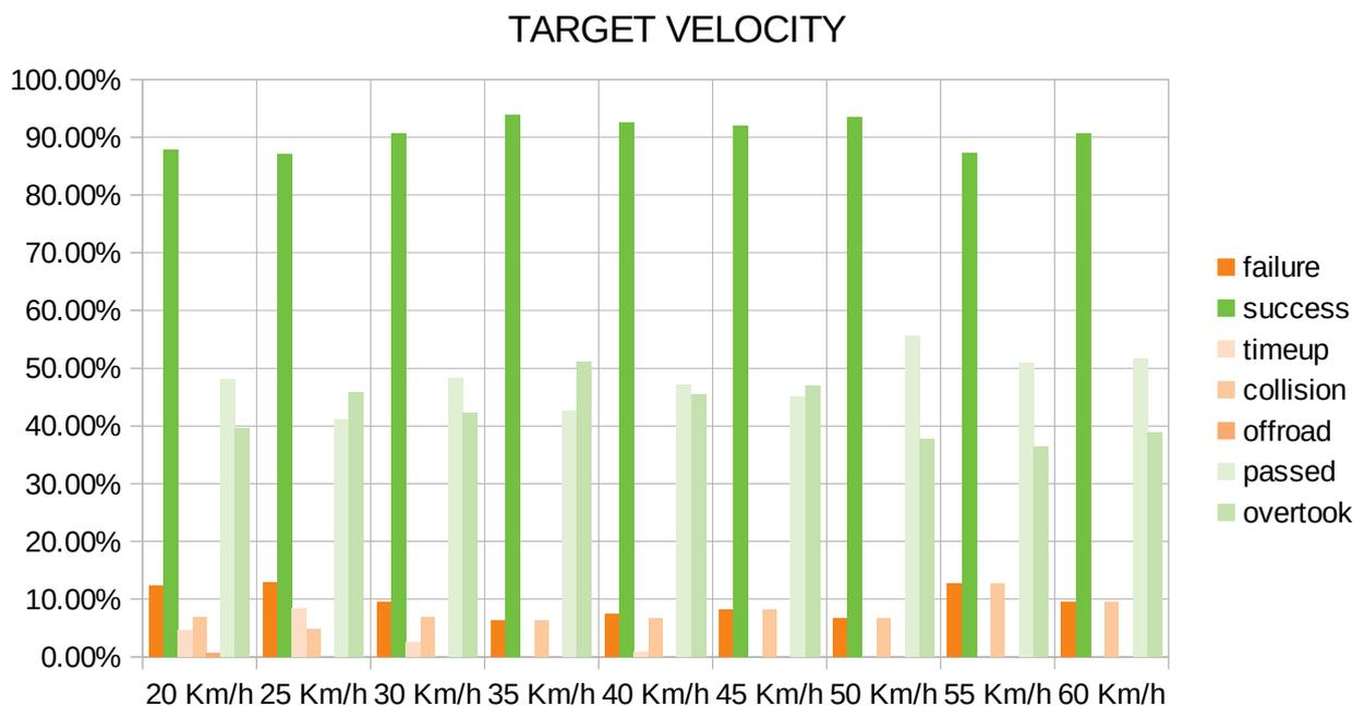
Figure 5.13 Results of Autonomous Emergency Steering Test – Target Velocity
