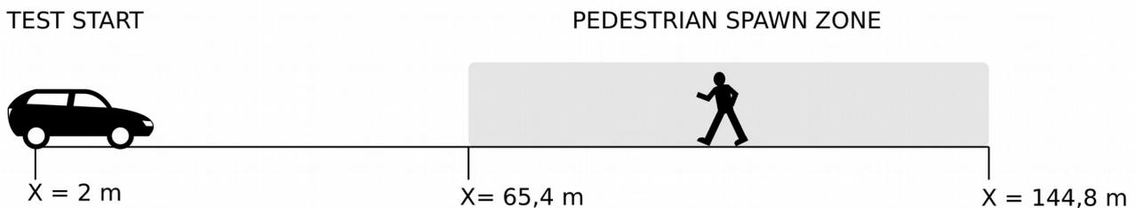
Figure 4.6 Autonomous Emergency Braking test Spawning Positions
