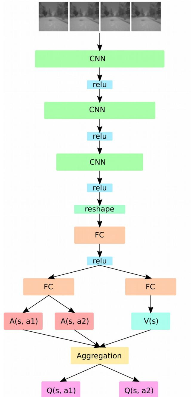
Figure 4.7 Autonomous Emergency Braking Neural Network
