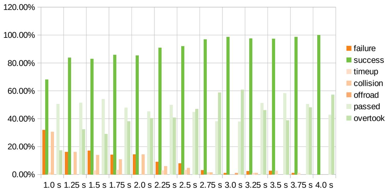
Figure 5.14 Results of Autonomous Emergency Steering Test – Time To Collision
