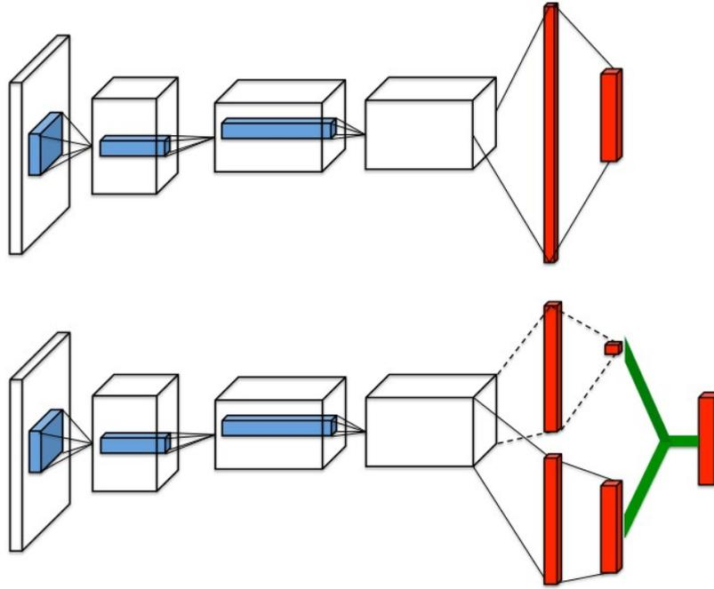
Figure 2.8 Standard Network (above) Dueling Network (below) [10]
