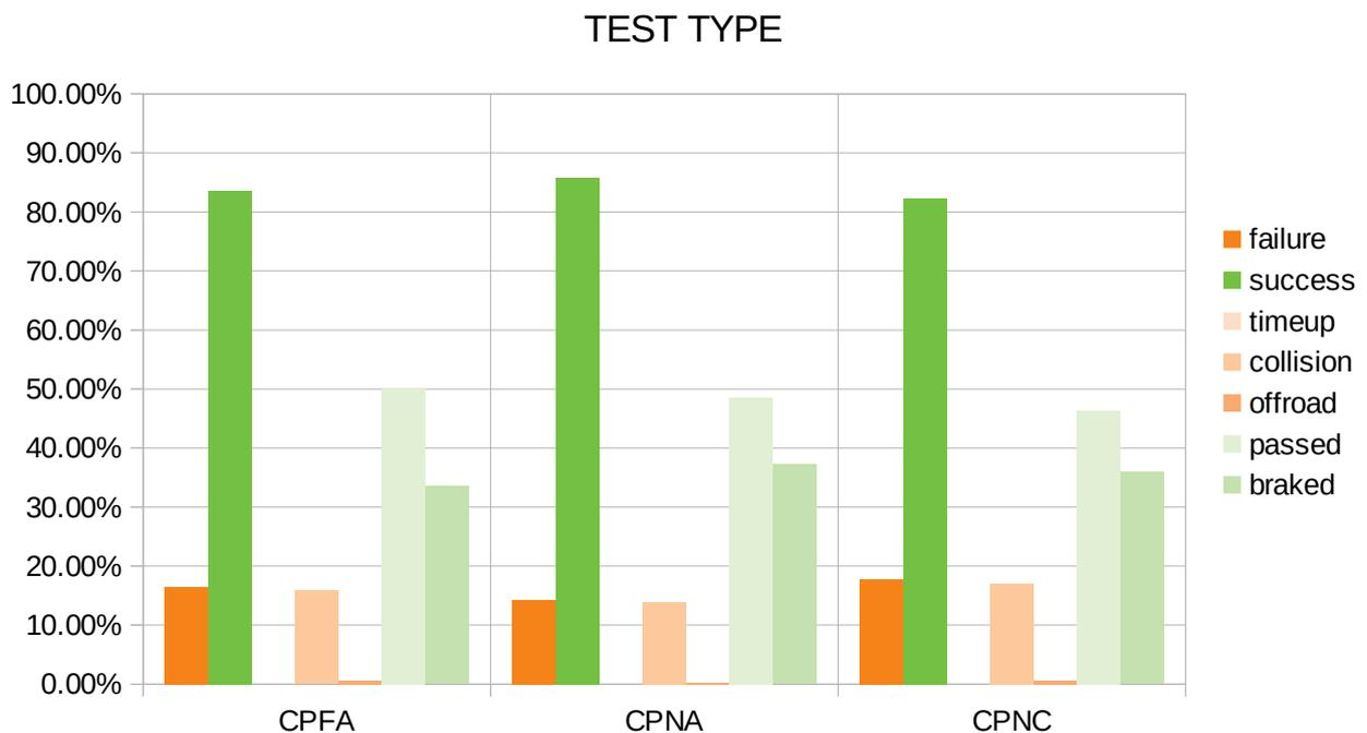
Figure 5.4 Results of Autonomous Emergency Braking Test – Test Type
