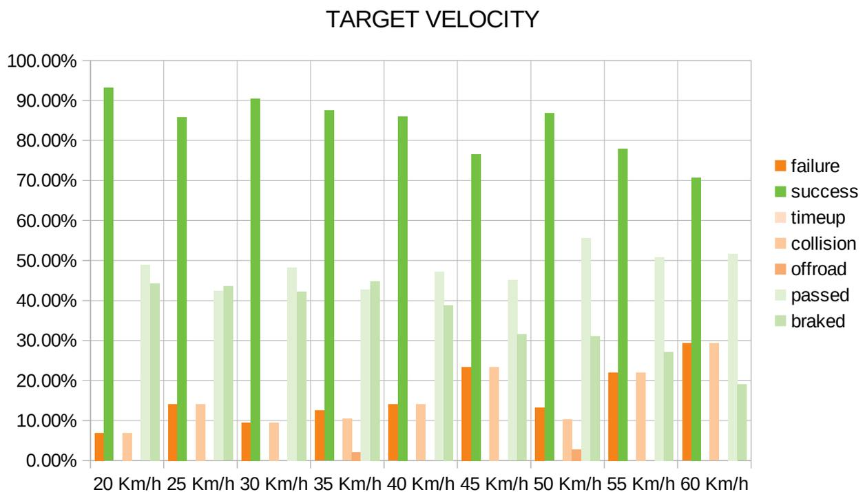
Figure 5.6 Results of Autonomous Emergency Braking Test – Target Velocity
