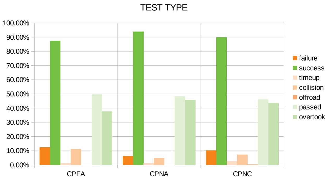
Figure 5.11 Results of Autonomous Emergency Steering Test – Test Type
