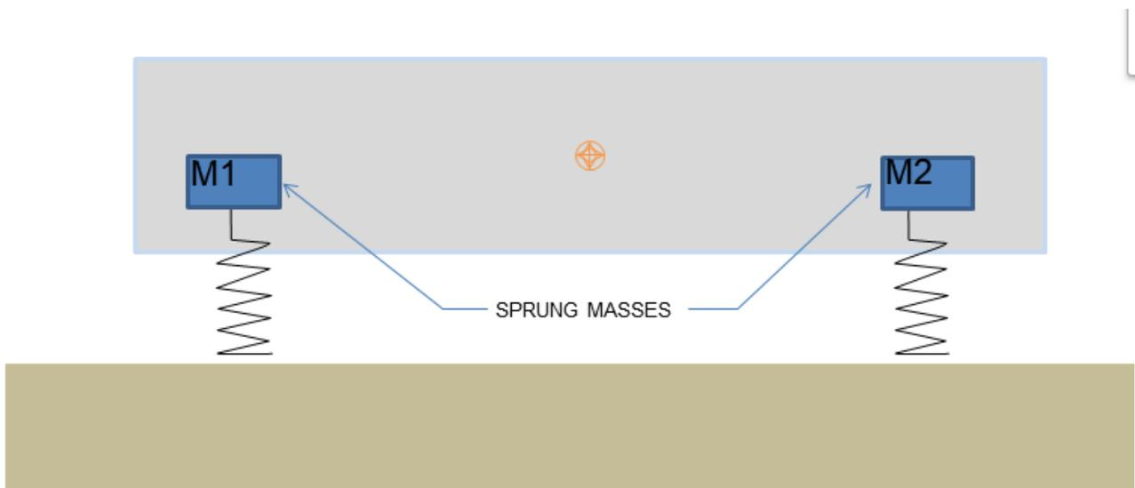
Figure 3.4 Vehicle representation as a collection of sprung masses of mass  $M1$  and  $M2$  [33]
