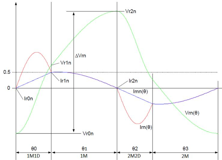
Figure 4.10: Normalised waveforms example (ZCS border:  $m = 2.6$ ,  $l_m = 7$ ,  $\Delta V_{rn} = 3.88$ )
