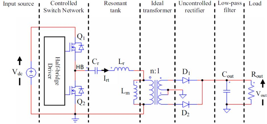
Figure 2.11: Detailed blocks cascade in the case of LLC converters
