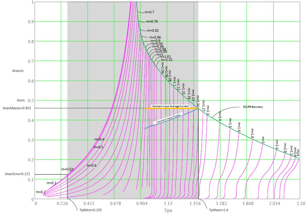
Figure 4.14: Plot of  $I_{inavno}$  as a function of  $T_{pn}$  for different values of  $\Delta V_{rn}$  (pink curves)
