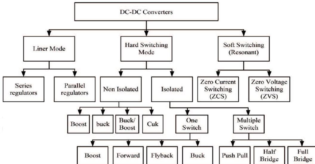
Figure 2.4: Classification of DC-DC converters
