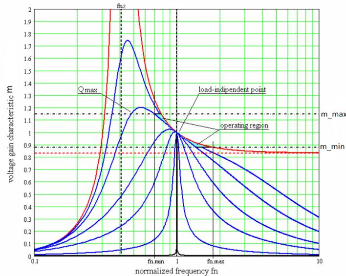
Figure 3.8: Operating region of the LLC converter in the voltage gain characteristic
