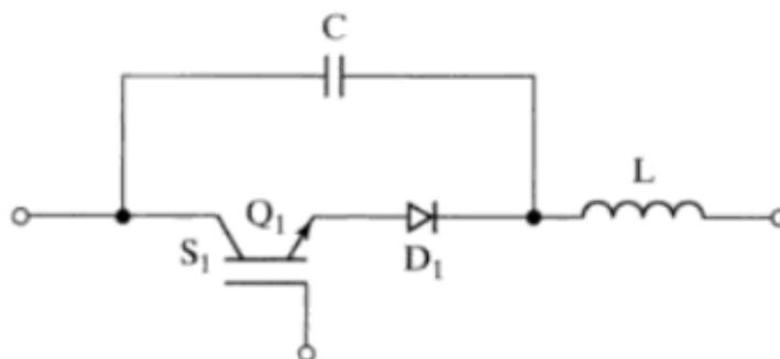
Figure 2.6: Example of a resonant switch
