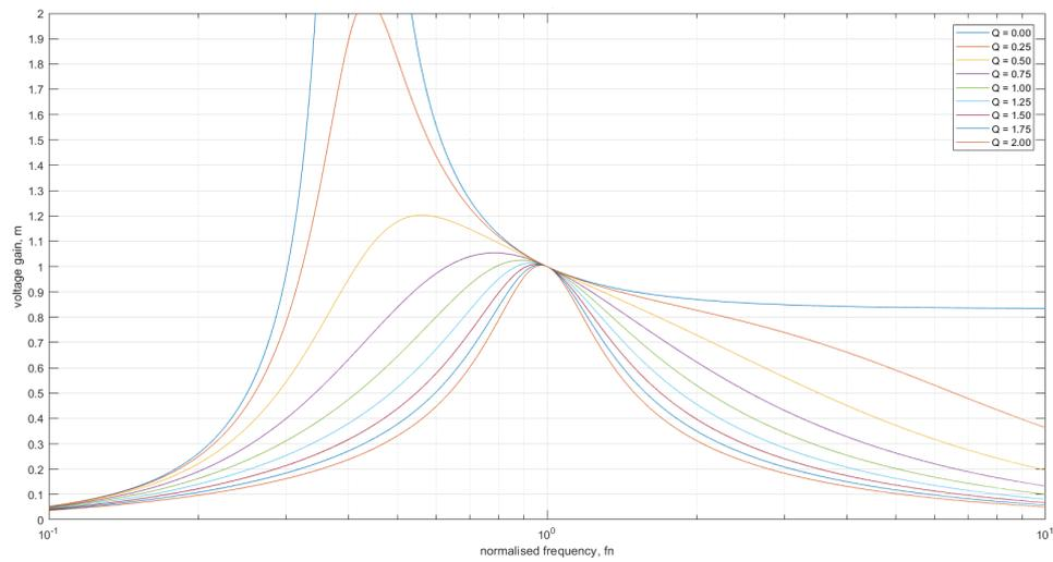
Figure 3.4: Voltage gain characteristics for different values of  $Q$  and  $l_m = 5$
