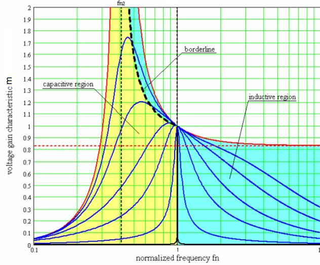
Figure 3.7: Inductive and capacitive regions in the voltage gain characteristic
