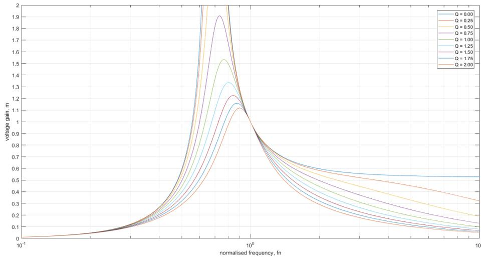
Figure 3.5: Voltage gain characteristics for different values of  $Q$  and  $l_m = 1.1$
