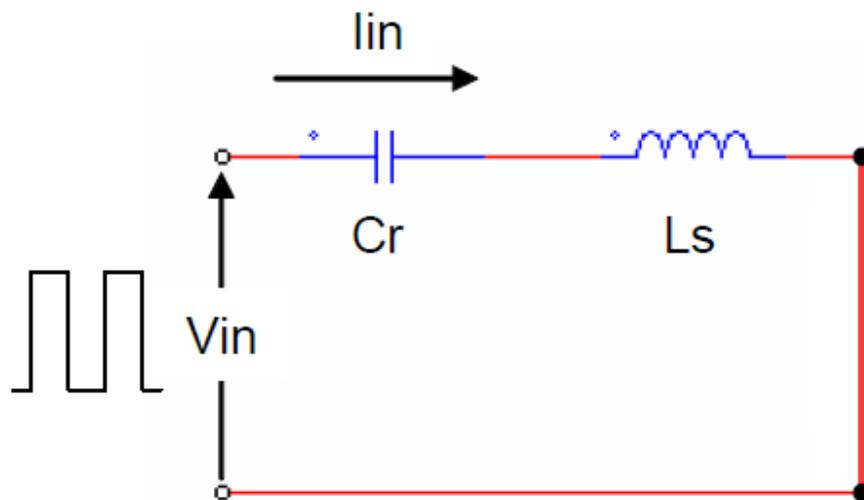
Figure 2.17: Circuit schematic in the case of short-circuit load
