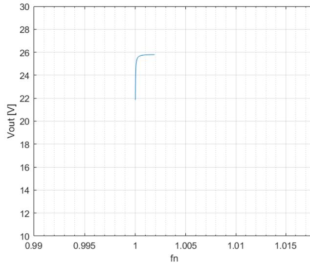
Figure 5.6: RHP border of the lossy LLC ( $R_M = 0.1 \Omega$  and  $R_D = 0.01 \Omega$ )
