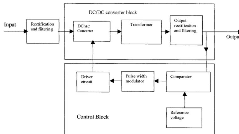
Figure 2.3: Block diagram of a voltage regulator
