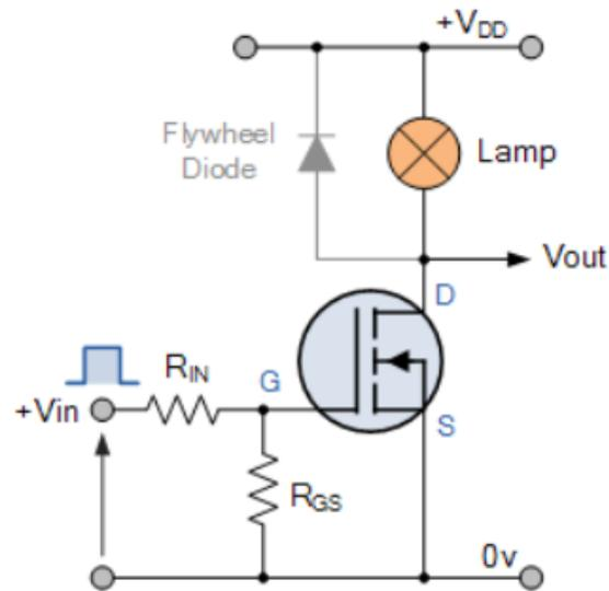
Figure 2.2: Switching circuit for the driving a resistive load
