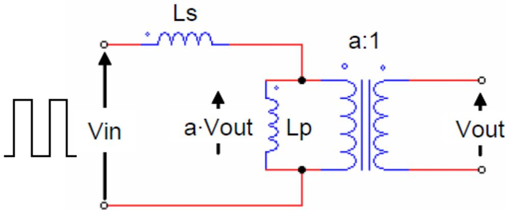
Figure 2.16: Circuit schematic in the case of open-circuit load
