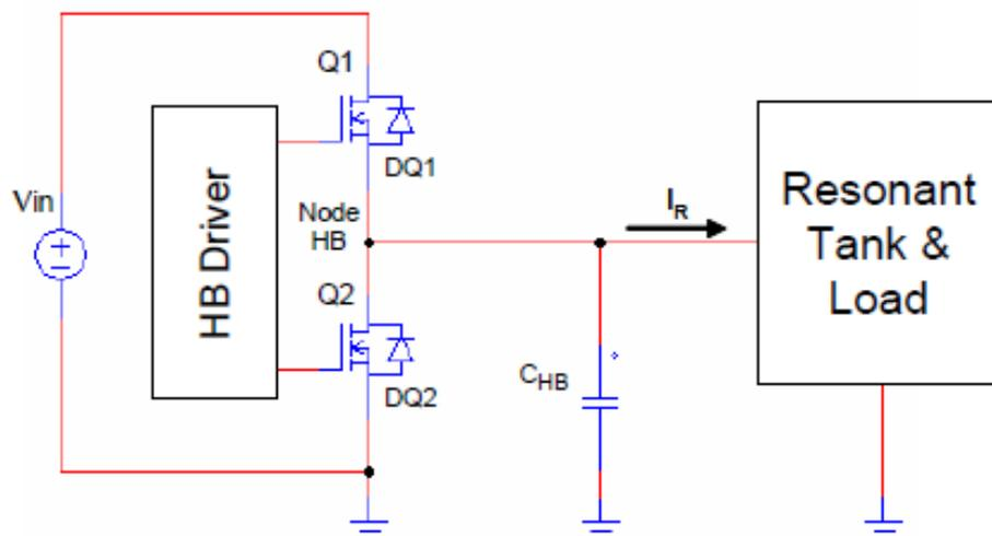
Figure 2.14: Reference scheme for the study of the switching mechanism
