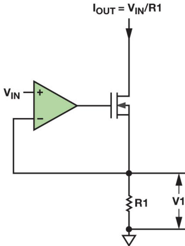
Figure 2.1: Circuit for current control through the use of a MOSFET working in saturation
