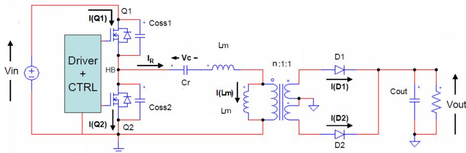
Figure 2.15: LLC reference schematic for the analysis of main operating regions
