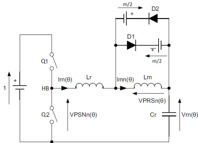
Figure 4.2: LLC converter normalised APR equivalent circuit
