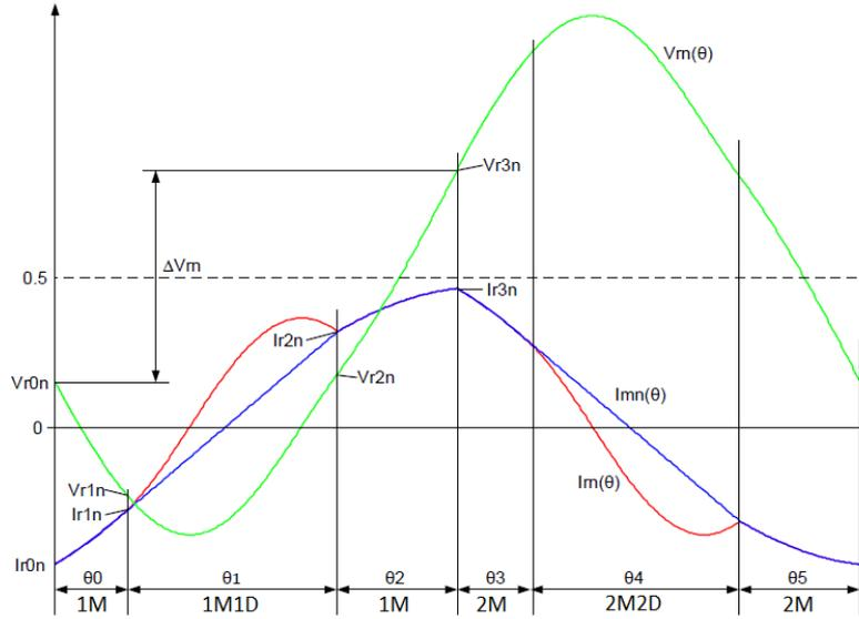
Figure 4.8: Normalised waveforms example (BRLP region:  $m = 2$ ,  $l_m = 5$ ,  $\Delta V_{rn} = 0.7$ )
