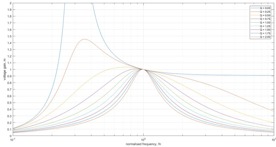
Figure 3.3: Voltage gain characteristics for different values of  $Q$  and  $l_m = 10$
