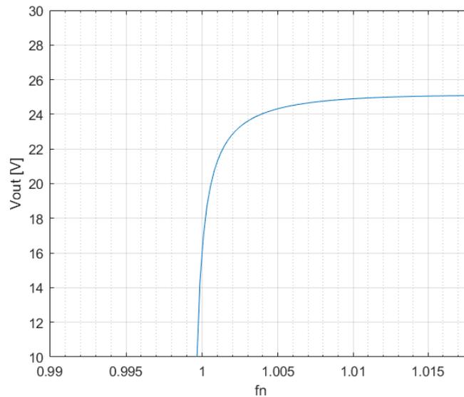
Figure 5.5: RHP border of the lossy LLC ( $R_M = 1$   $\Omega$  and  $R_D = 0.1$   $\Omega$ )
