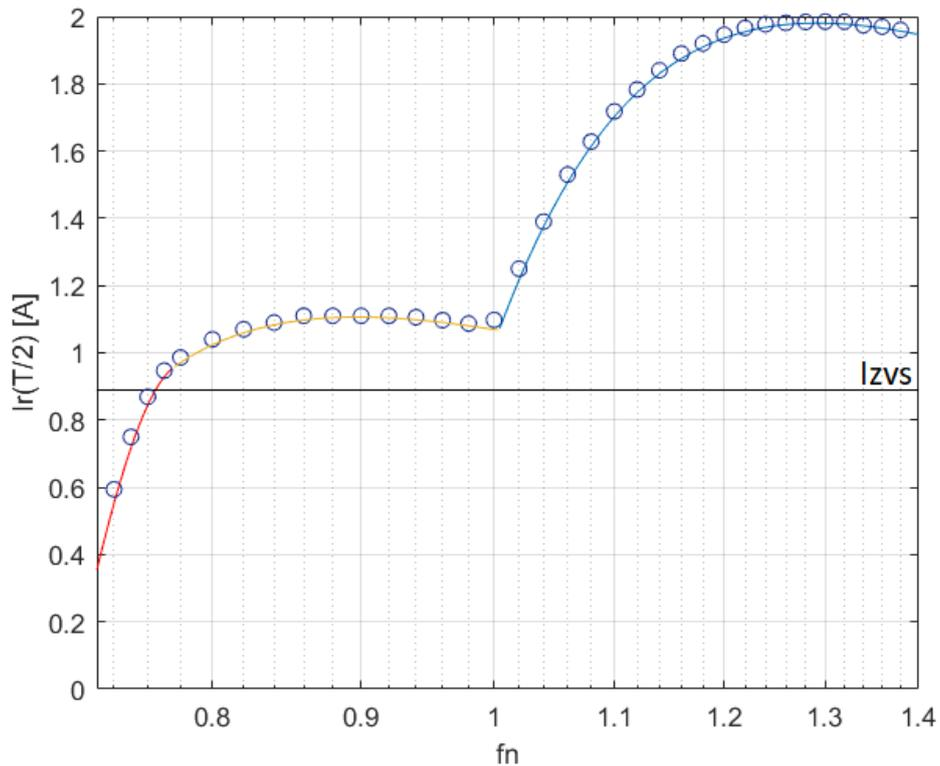
Figure 5.11: Trend of  $I_r(T/2)$  as a function of the normalised frequency
