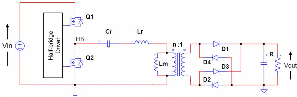
Figure 3.1: LLC starting schematic for the FHA analysis
