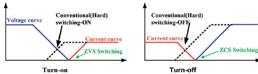
Figure 2.5: Current and voltage waveforms of hard-switching and soft-switching
