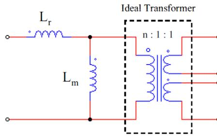
Figure 2.12: APR model of the lossless transformer
