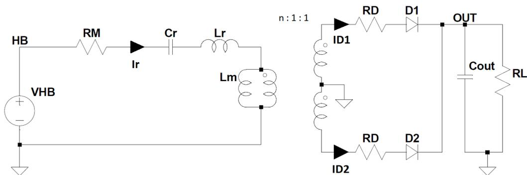
Figure 5.1: Lossy LLC schematic under the assumption of zero dead-time
