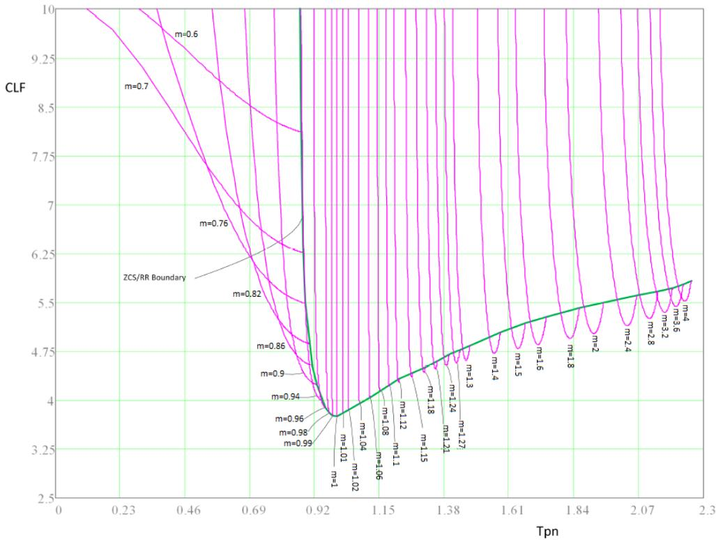
Figure 4.12: Plot of CLF as a function of normalised switching period ( $T_{pn} = T/T_r$ ) for different values of  $\Delta V_{rn}$  (pink curves) and  $l_m = 5$
