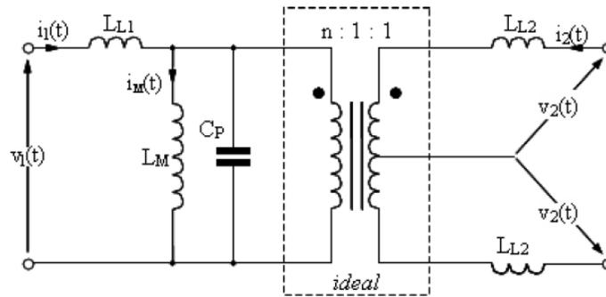
Figure 2.19: Equivalent schematic of a transformer including self-resonance capacitor
