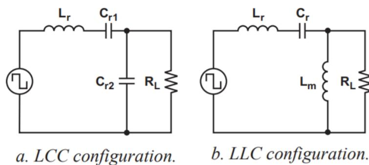
Figure 2.9: Basic hybrid load resonant converters
