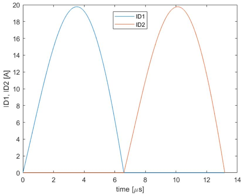
Figure 5.4: Example of the periodic evolution of  $I_{D1}$  and  $I_{D2}$
