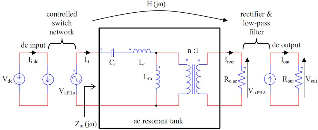
Figure 3.2: Linearised model of the LLC under the FHA
