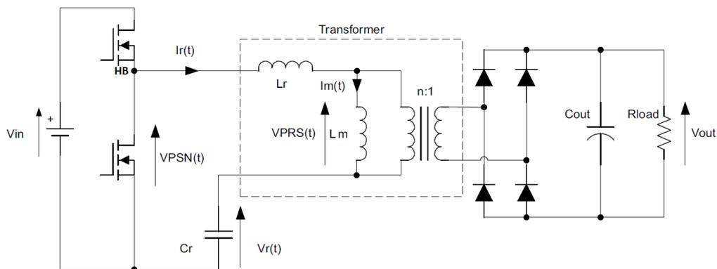
Figure 4.1: LLC converter schematic
