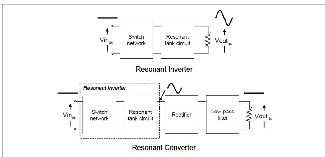
Figure 2.7: General block scheme of a resonant tank converter
