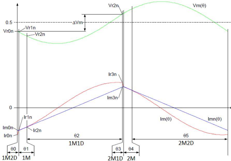
Figure 4.6: Normalised waveforms example (ARLP region:  $m = 0.94$ ,  $l_m = 5$ ,  $\Delta V_{rn} = 0.1$ )
