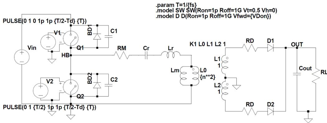
Figure 5.8: LTspice schematic of the complete lossy LLC converter
