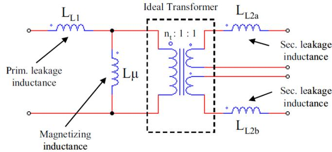
Figure 2.13: Physical model of the lossless transformer
