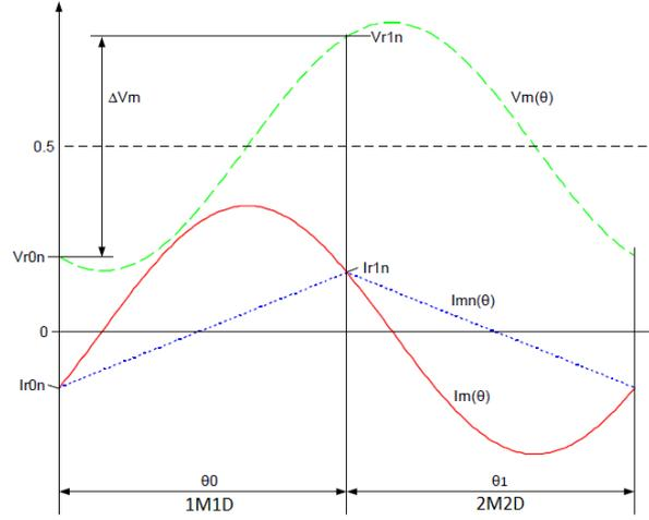
Figure 4.9: Normalised waveforms example (RHP boundary:  $m = 1, l_m = 5, \Delta V_{rn} = 0.6$ )
