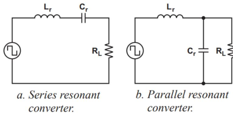
Figure 2.8: Basic series and parallel resonant converters
