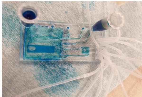
*Figure 55. Unsuccessful priming attempt, with internal bubbles still present*
