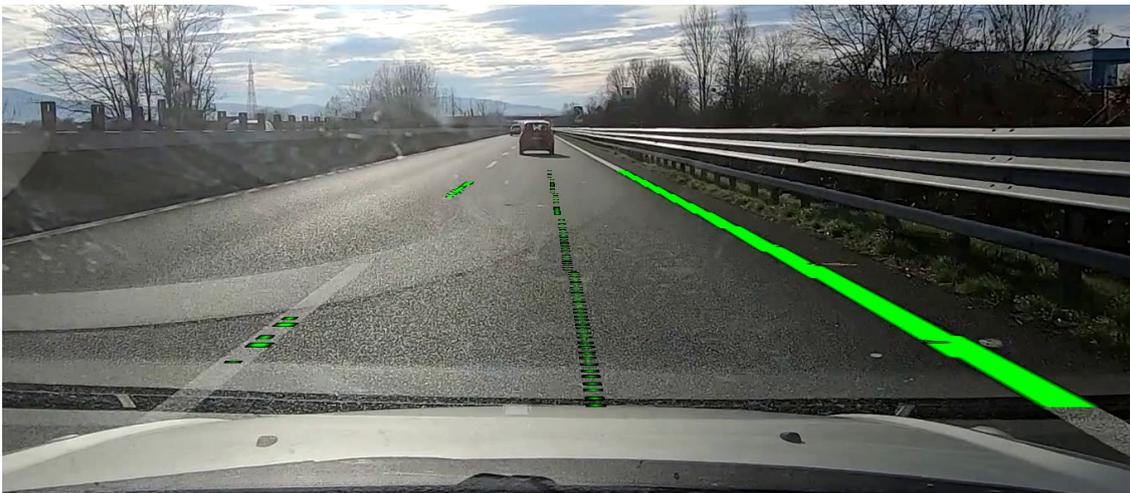
Figure 7.9. Example of problems caused by sun light in front of the camera - 1, Turin ring road
