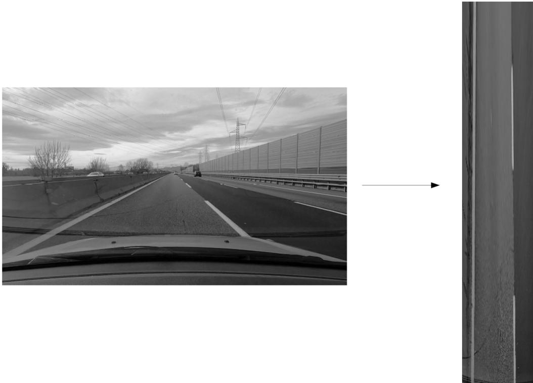
Figure 5.5. Example of the inverse-perspective mapping handled by the pre-processing thread
