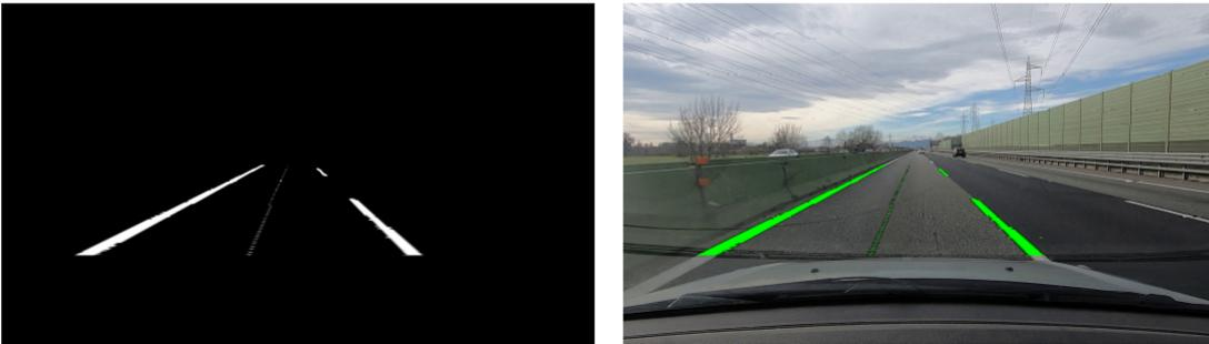
Figure 5.10. Example of the output frame composition handled by the output thread
