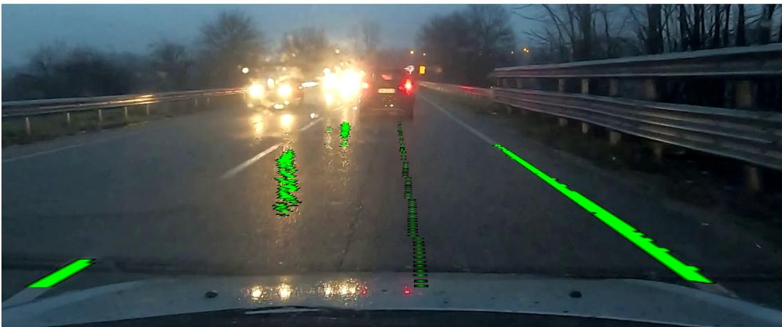
Figure 7.15. Example of problems caused by rain - bad detection due to light reflection on the road, Orbassano (TO)
