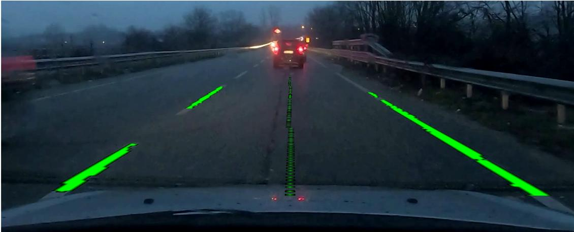
Figure 7.14. Example of problems caused by rain - good detection in absence of incoming cars, Orbassano (TO)
