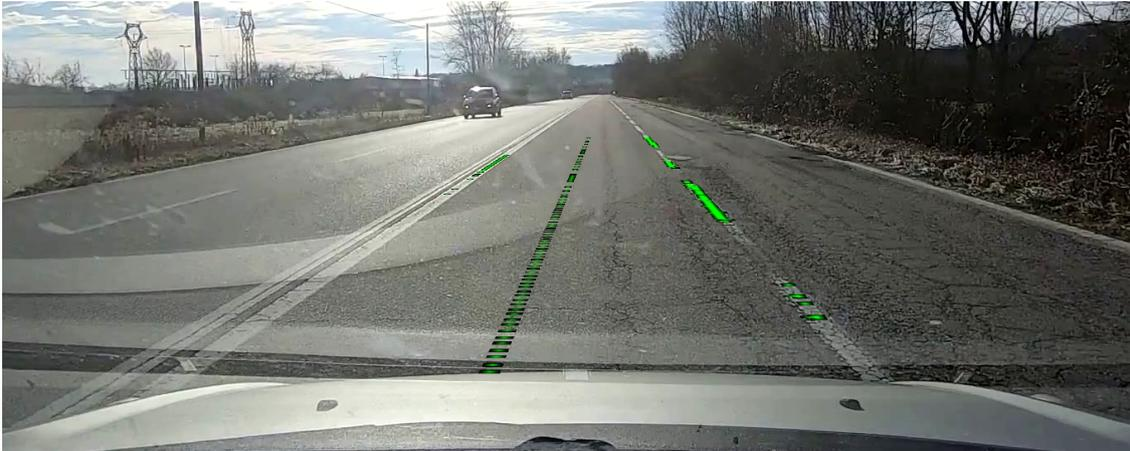
Figure 7.10. Example of problems caused by sun light in front of the camera - 2, Busano (TO)
