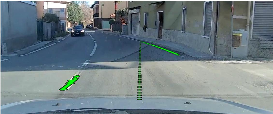
Figure 7.21. Example of erroneous road model fitting, Rivara (TO)
