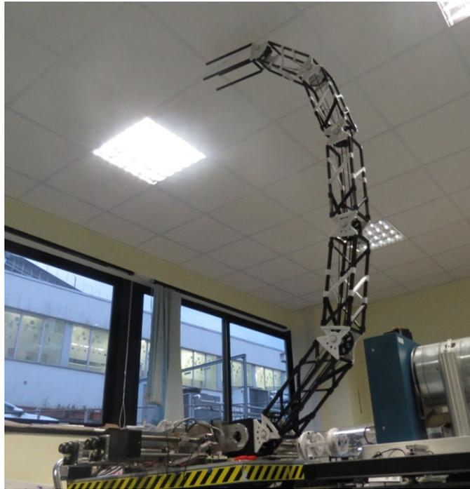
Figure 1.7: An image of snake-arm robot prototype composed by 6 revolute joints
