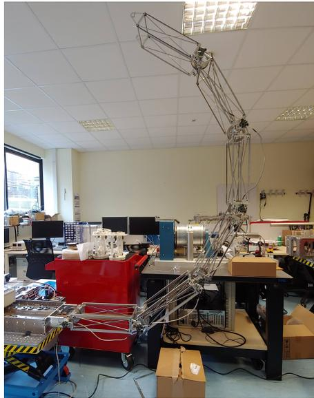
Figure 5.1: The 6 revolute joints robot prototype used for experiments
