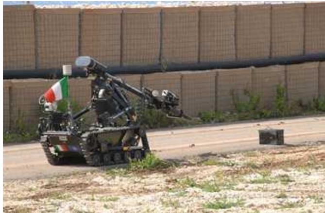
Figure 1.3: The heelbarrow Mk8 plus used by Italian Army as bomb disposal unit
