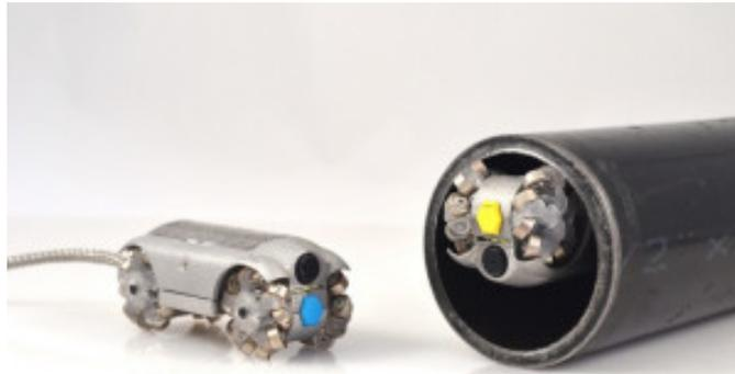
Figure 1.5: HoneyBee pipe inspection robot sliding through a small diameter pipe by means of its mecanum magnetic wheels.
