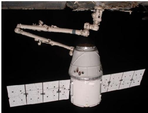
Figure 2.1: Berthing operation schematic and the Canadarm2 manipulator of the ISS grappling a Dragon spacecraft (credit: NASA)
