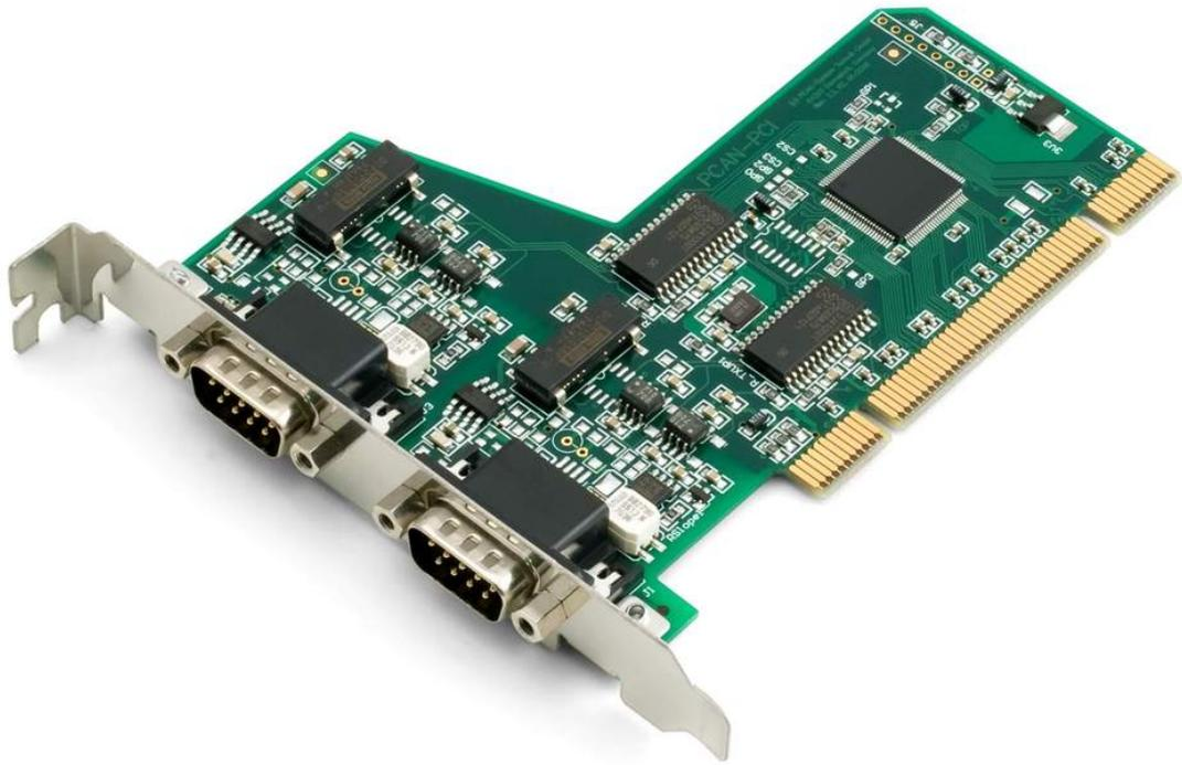
Figure 5.5: PCI to CAN adapter
