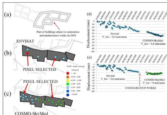
Figure 24: Behavior of buildings aggregate before and after the rehabilitation works occurred in 2010, (Infante, et al., 2014).
