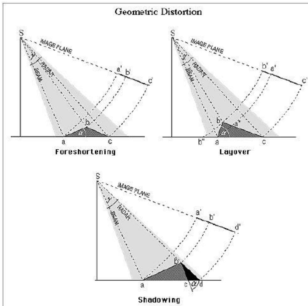
Figure 3: Perspective deformations in SAR image, (Tele-Rilevamento Europa T.R.E. s.r.l., 2009).
