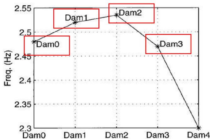
Figure 47: Frequency/level of damage graph of the bridge, (Sohn, et al., 2002).
