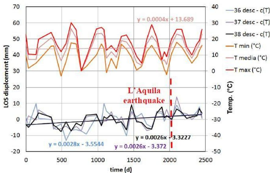
Figure 28: Displacements on Line Of Sight (LOS) direction in the south nave near the transept after removing thermal contribution, (De Canio, et al., 2015).
