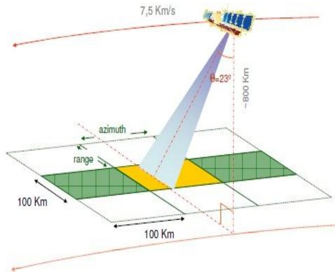
Figure 1: Acquisition geometry of the SAR ERS-1 system, (Tele-Rilevamento Europa T.R.E. s.r.l., 2009).
