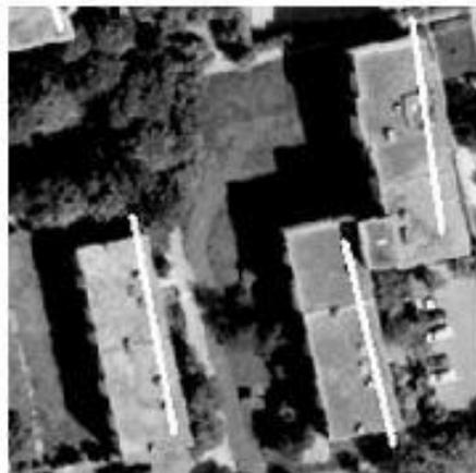
Figure 49: Optical data and extracted corner lines from InSAR data, (Wegner, et al., 2011).
