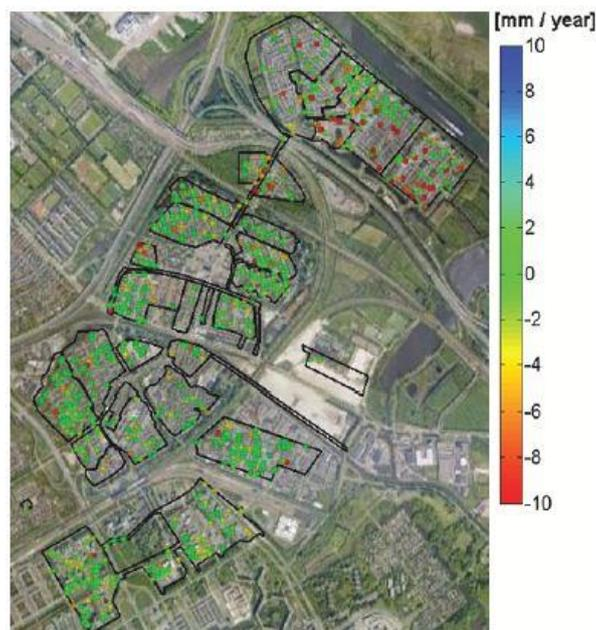
Figure 54: PS deformation of the Diemen region, (Dheenathayalan, et al., 2011).
