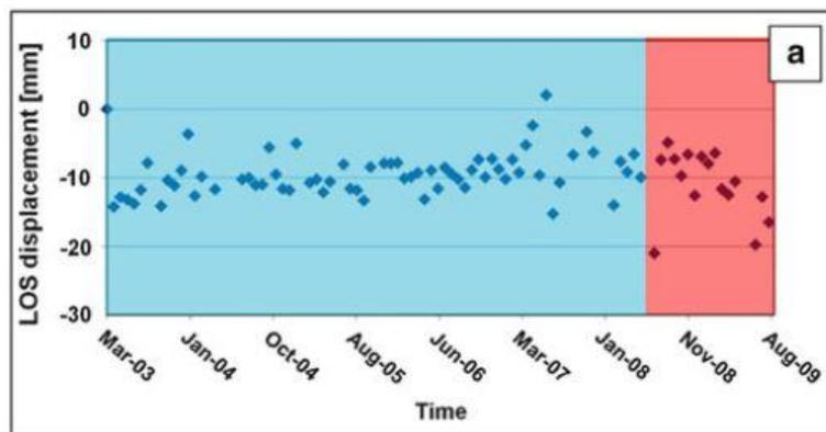
Figure 69: Time series of deformation identified in the NW corner of the Nero's Golden House, Oppian Hill, (Tapete, et al., 2013).
