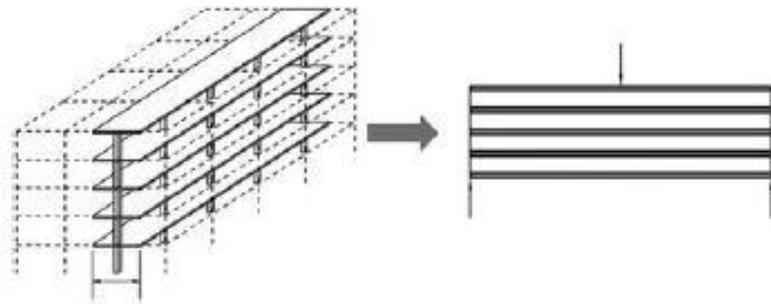
Figure 25: Equivalent beam scheme, (Arangio, et al., 2013).
