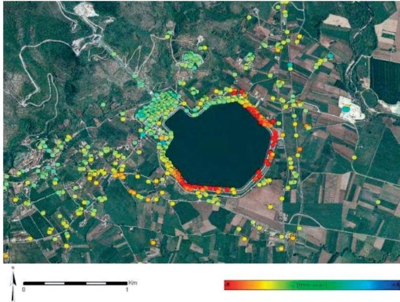
Figure 10: Permanent Scatterer analysis superimposed to an optical photo, (Reg. Liguria, Reg. Piemonte, Reg. Valle D'Aosta, 2009)
