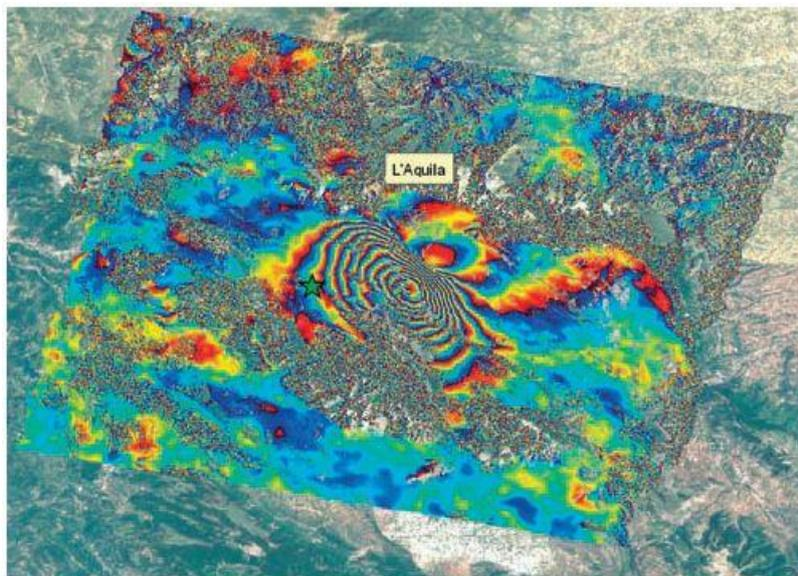
Figure 4: Interferogram generated from two different SAR Images in the city of L'Aquila, (Reg. Liguria, Reg. Piemonte, Reg. Valle D'Aosta, 2009).
