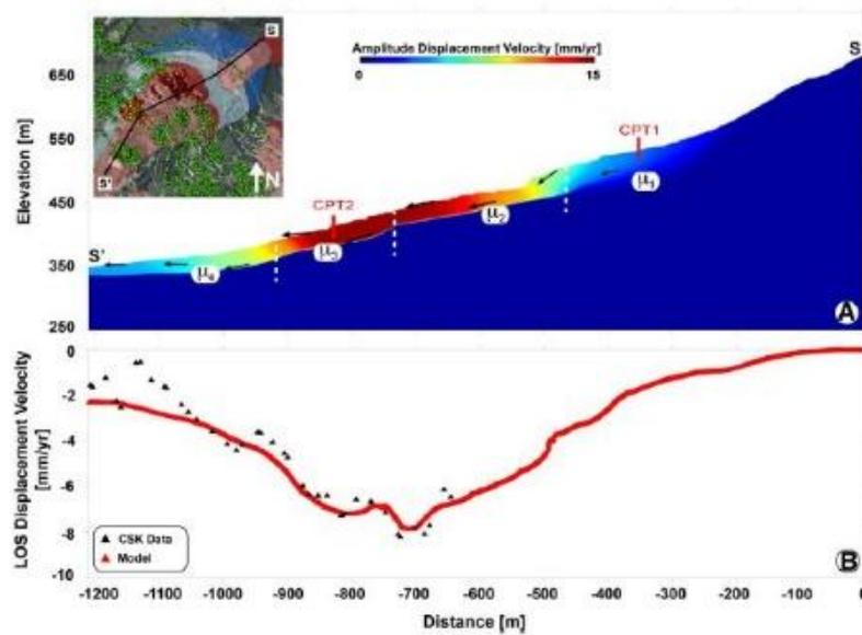
Figure 34: Displacements from SAR and FEM analysis, (Calò, et al., 2014).
