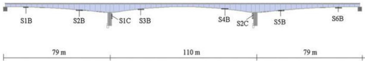
Figure 58: Sensors location on the three spans of box girder bridge model, (Suryanita & Adnan, 2013).
