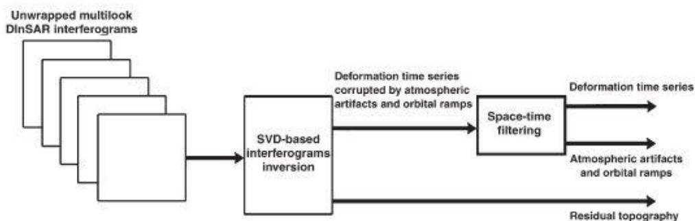
Figure 14: SBAS method steps, (Casu, et al., 2006).
