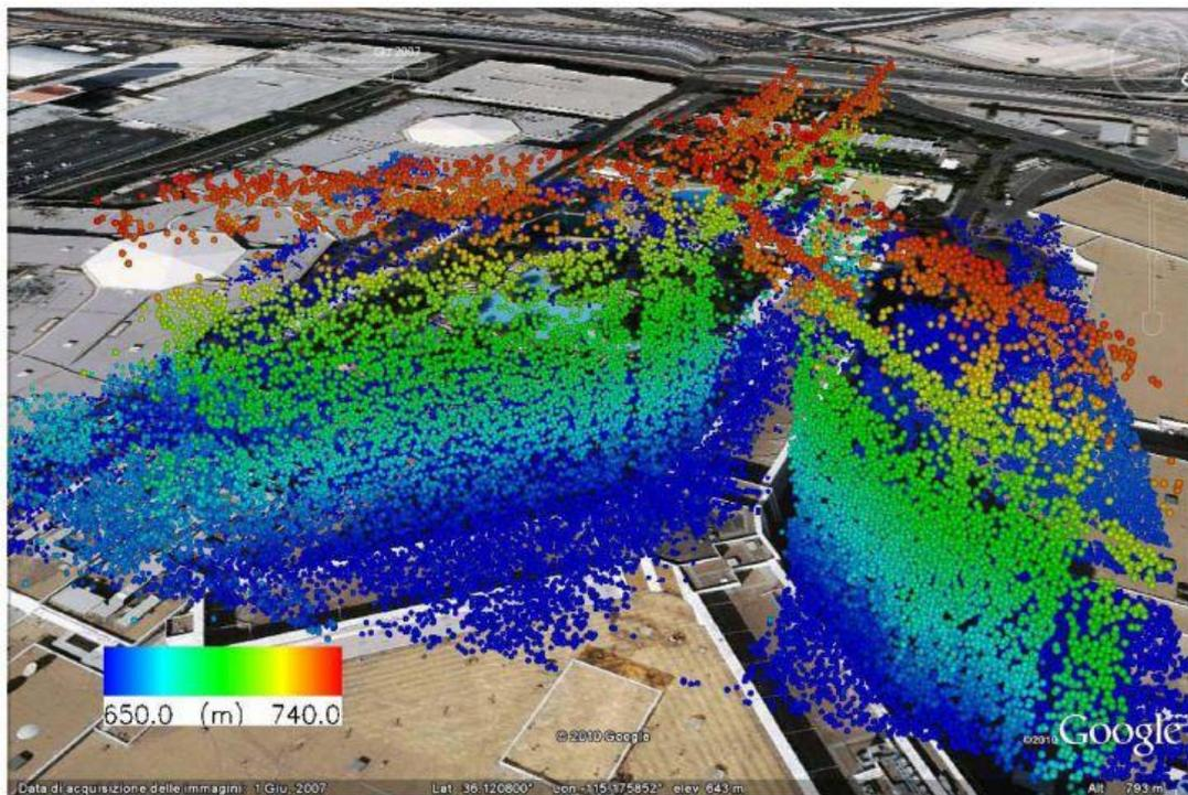
Figure 19: Three-dimensional view derived from scatterers with SAR tomography on Google Earth, (Reale, et al., 2011).
