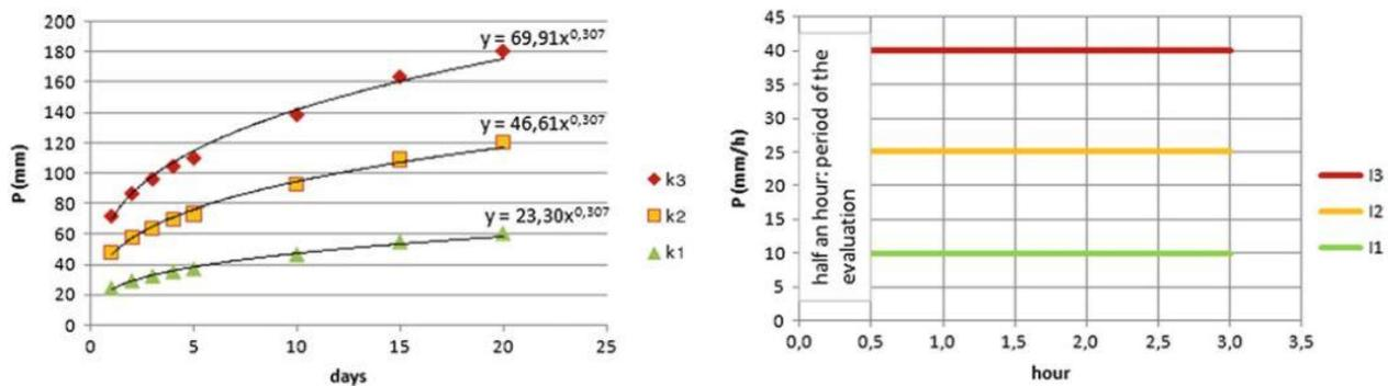
Figure 65: : Threshold equations due to cumulative rainfall (left), thresholds related to rain intensity (right), (Basile & Panebianco , 2013)
