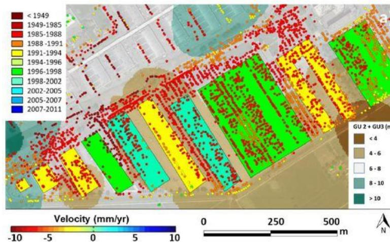
Figure 18: Velocity of persistent scatterers of COSMO-SkyMed over a thickness map of compressible soils, (Bozzano, et al., 2018).
