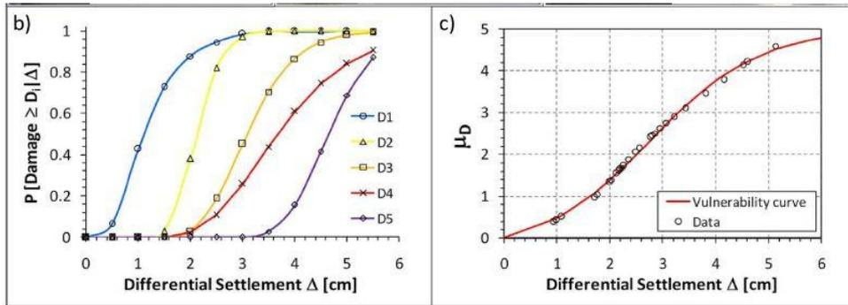
Figure 23: (b) fragility curves, (c) vulnerability curves for masonry buildings in Lungro, (Peduto, et al., 2018).
