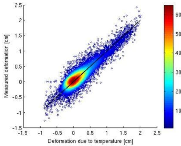
Figure 37: Thermal deformation measured by SAR data and simulated thermal dilatation, (Fornaro, et al., 2013).
