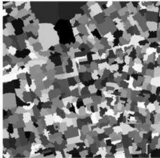
Figure 50: Segmentation of the optical image, (Wegner, et al., 2011).
