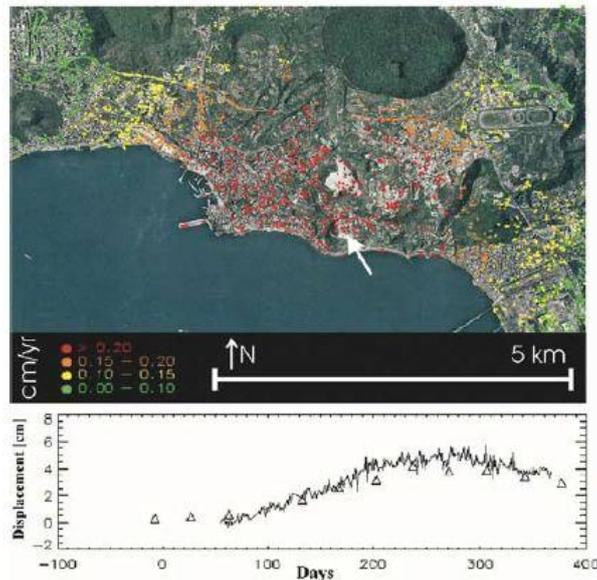
Figure 15: Comparison between GPS and SAR data in Campi Flegrei area, (Berardino, et al., 2002).
