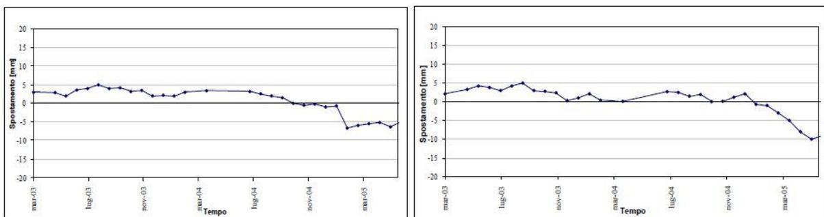
Figure 70: Examples of anomalies trend deformation: High deformation (left), acceleration of deformation (right), (Cigna, 2010).
