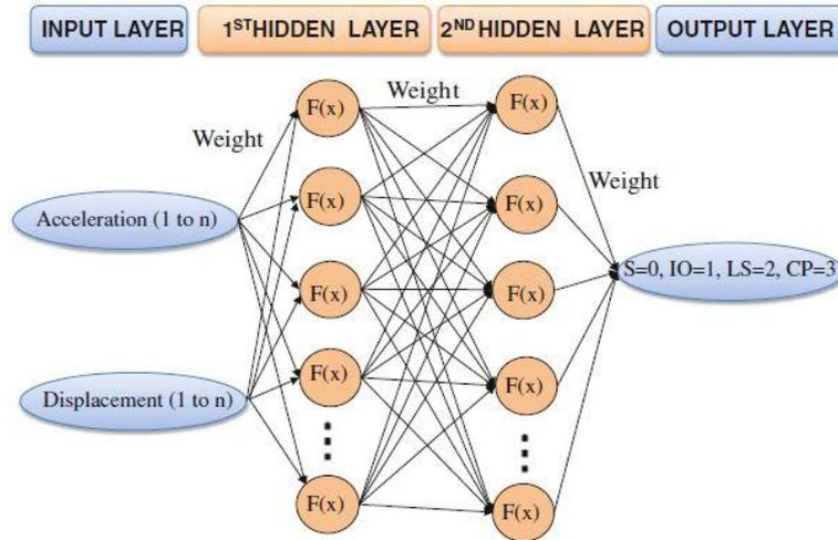
Figure 59: neural networks structure for the early-warning system, (Suryanita & Adnan, 2013).
