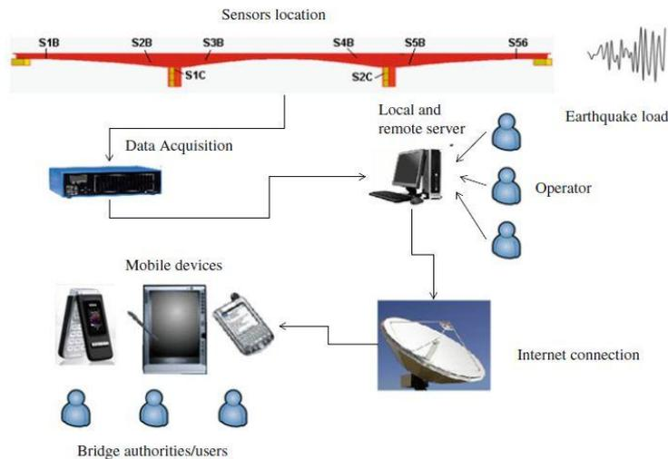
Figure 61: The bridge monitoring system, colours indicate level of damage in the structure, (Suryanita & Adnan, 2013).
