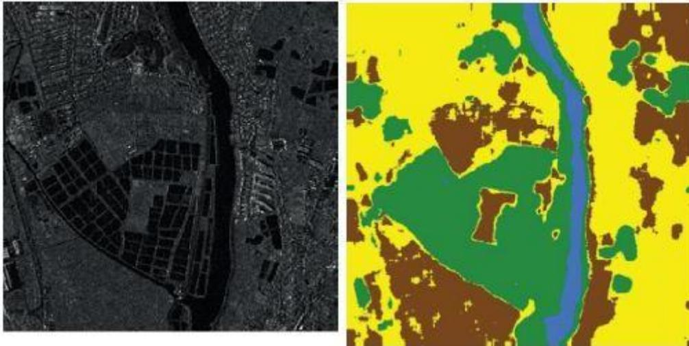
Figure 53: : (left) SAR image of Foshan (China), (Right) Results of SVM method with alpha stable distribution: buildings (yellow), river (blue), marsh (green), farmland (brown), (Peng, et al., 2011).
