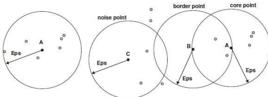
Figure 44: Core, border and noise points in DBSCAN method, (Anon., 2008).
