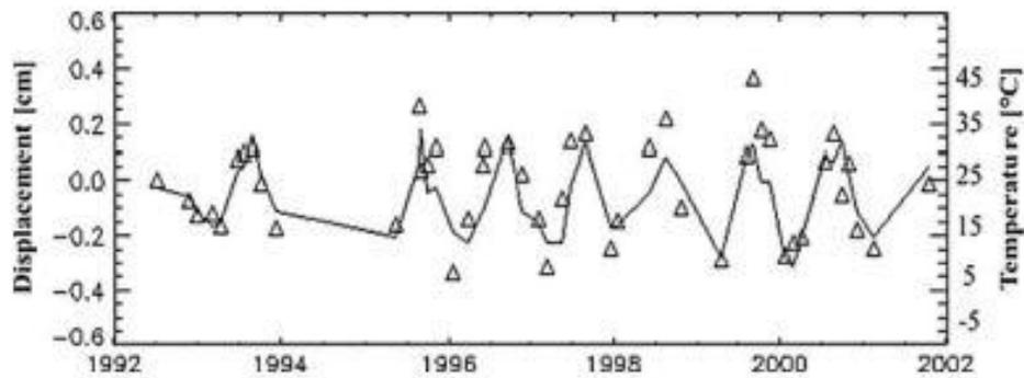
Figure 16: Overview between temperature and displacements data (triangles SAR data, continuous line temperature), (Berardino, et al., 2002).
