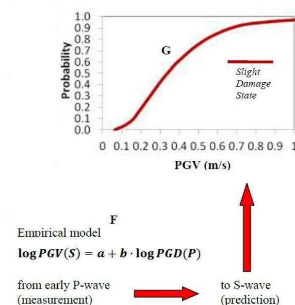
Figure 62: Prediction of the PGV for S-waves and example of derived fragility curve, (Megalooikonomou, et al., 2018).
