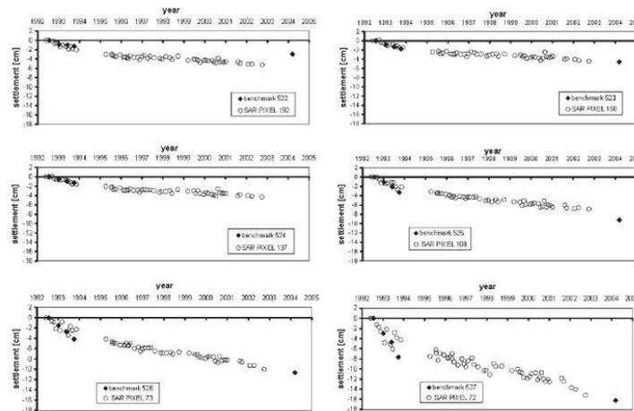
Figure 26: displacement comparison (from SAR and ground levelling data), (Cascini, et al., 2006).
