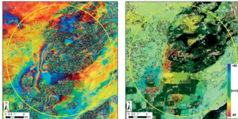
Figure 5: Deformation map generated from an interferogram, (Reg. Piemonte, Reg. Liguria, Reg. Valle D'aosta, 2012)
