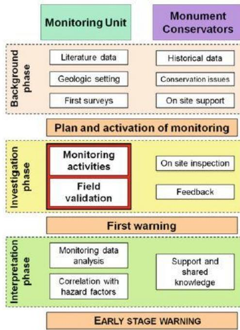
Figure 68: Flow chart of the 'early stage warning', (Tapete, et al., 2013).
