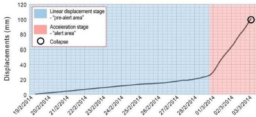
Figure 73: Displacements toward the sensor measured along the LOS, (Pratesi, et al., 2015).
