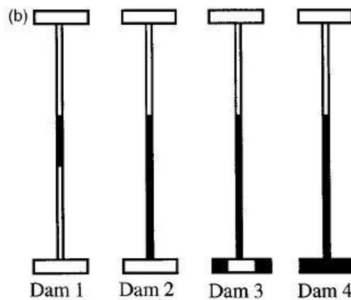
Figure 46: four sections damaged considered in the bridge (black area represents reduced cross section), (Sohn, et al., 2002).
