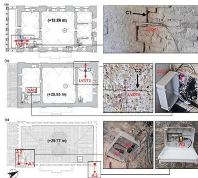
Figure 27: Static monitoring system: (a) LVDT1 in the south façade, (b) LVDT2 in the main crack of the north façade, (c) piezometric accelerometers on the roof of the palace, (Cavalagli, et al., 2019).
