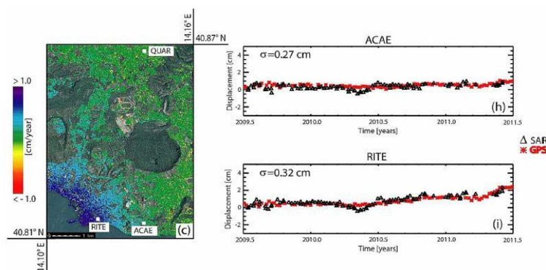
Figure 17: Comparison between SAR and GPS measurements in Campi Flegrei area, (Bonano, et al., 2013).
