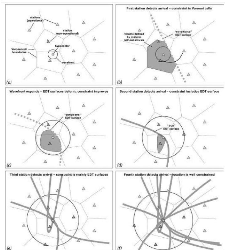
Figure 57: Steps for the evaluation of the earthquake hypocenter, (Satriano, et al., 2010)
