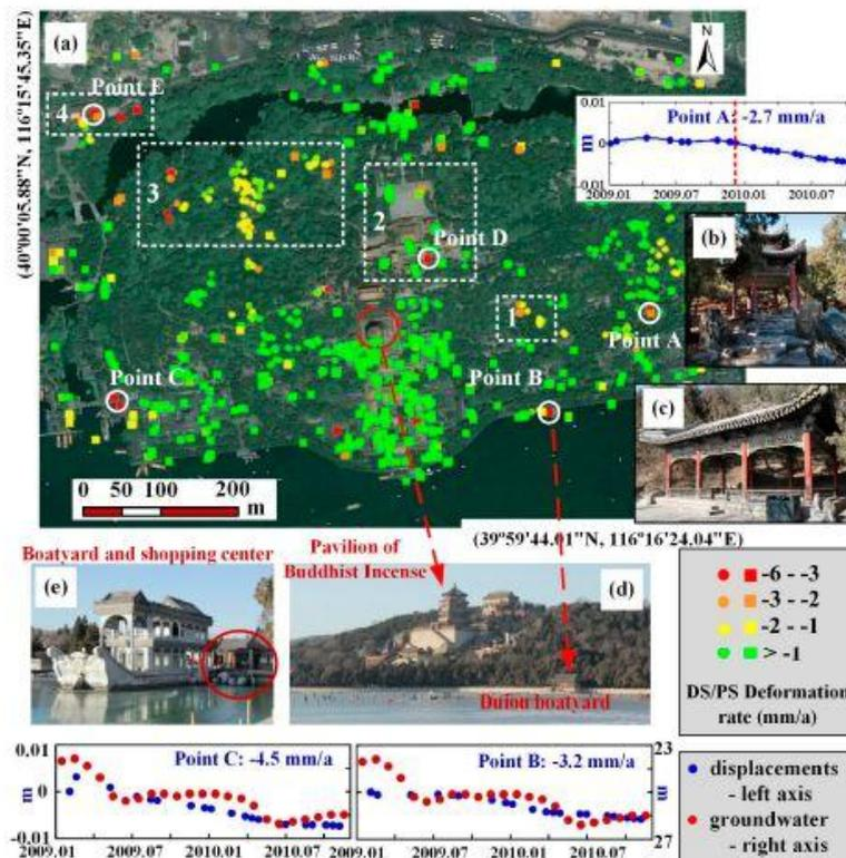
Figure 31: Map of deformations of the Longevity Hills and groundwater data used to validate motion evolutions of several points, (Tang, et al., 2016).
