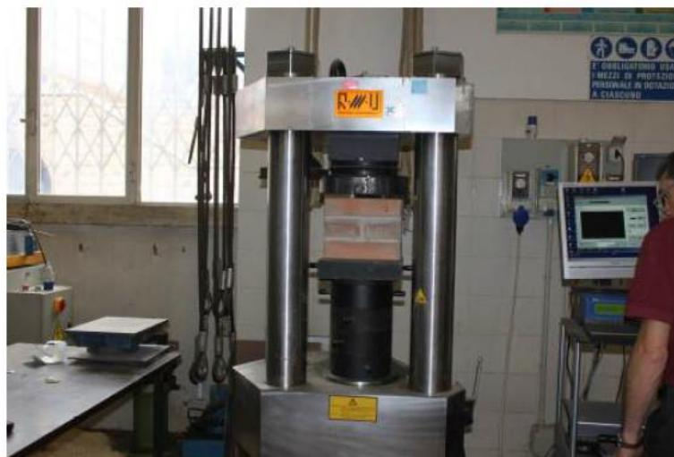
Figure 31 - Compressive test apparatus (DCPST laboratory).
