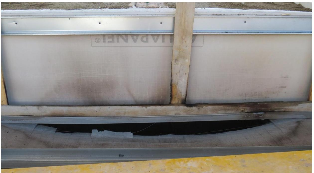
Figure 46 - Ignition of supporting structure.
