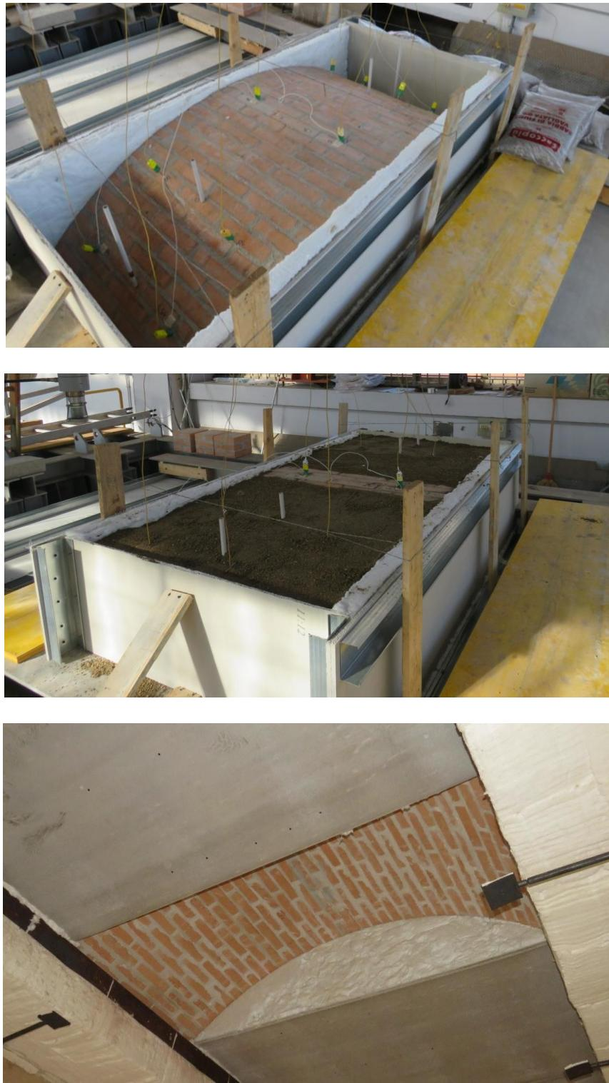
Figure 28 - Top, lateral, bottom views of arch and confinement for filler material and thermal insulation.
