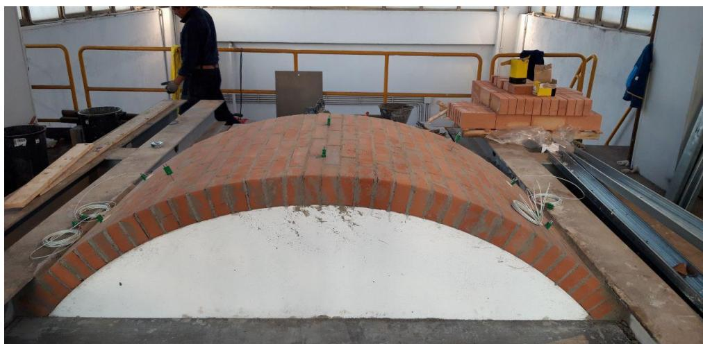
Figure 22 - Arch built for experimental test 1. Photo has been taken on the ceiling of the oven.
