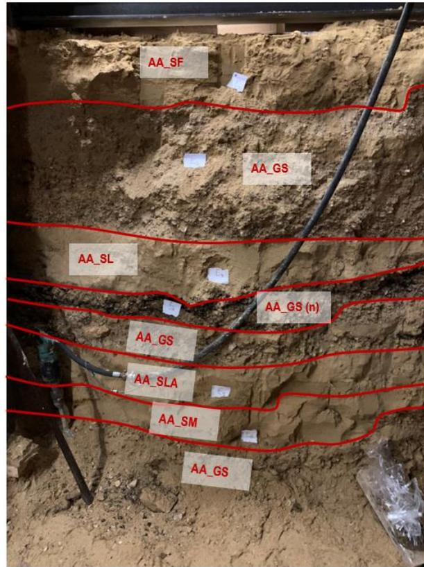
**Figure 4.1-1: Detail of the position of the samples taken - half right upper section (ENSER France, 2019)**
