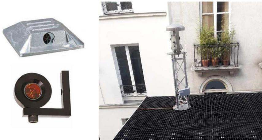
**Figure 5.3-26: Topographic targets and automatic theodolite on the metallic structure of Rue Duphot (Solexperts, 2019-2020)**
