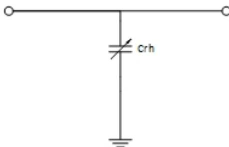
Figure 1.3: Right Heart electrical equivalent circuit
