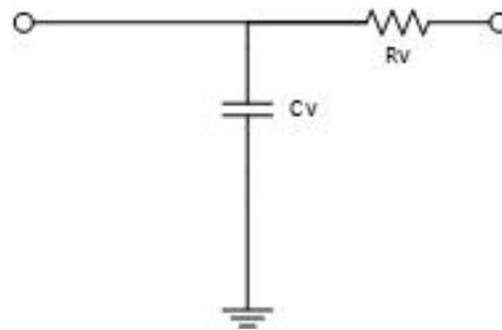
Figure 1.12: Veins electrical equivalent circuit
