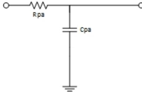
Figure 1.14: Pulmonary Arteries electrical equivalent circuit
