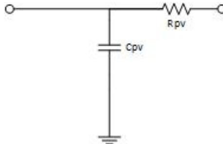
Figure 1.15: Pulmonary Veins electrical equivalent circuit
