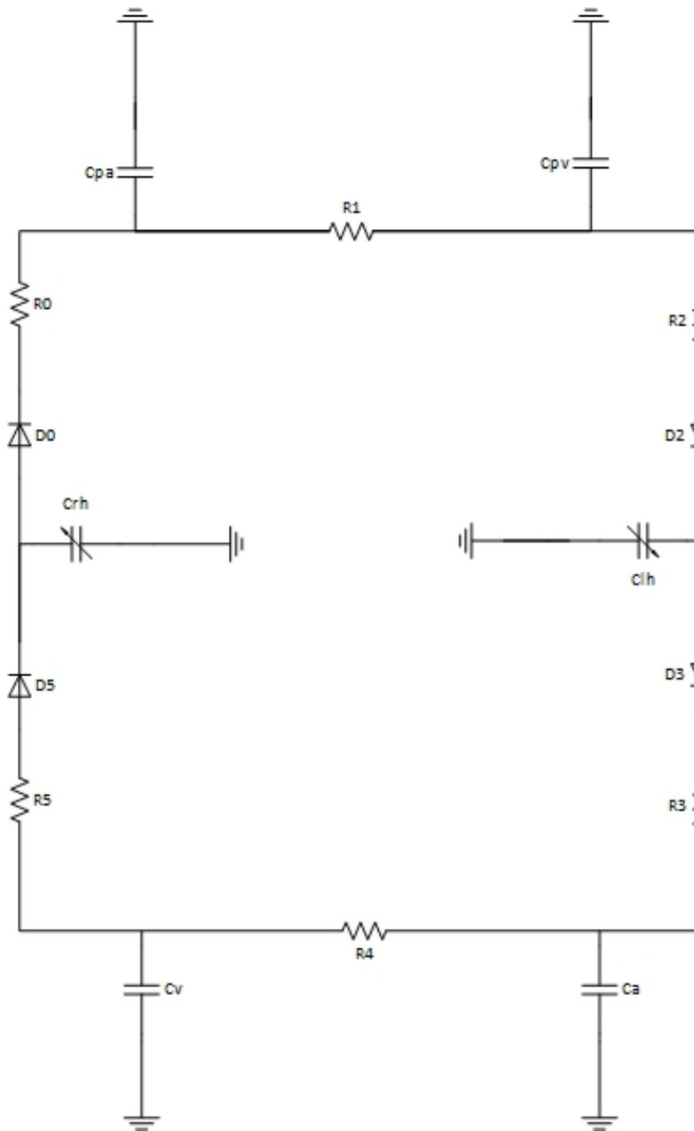
Figure 1.18: Six compartment model electrical equivalent circuit
