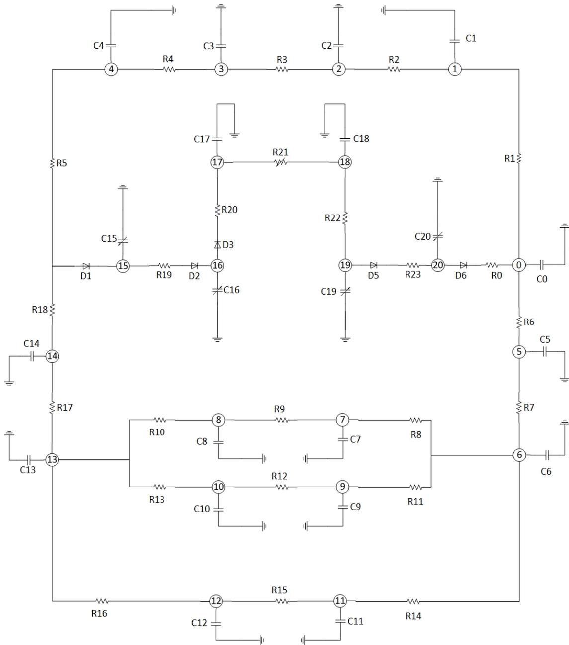
Figure 1.21: Twentyone Compartment Electrical Model
