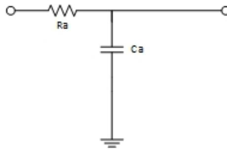
Figure 1.11: Arteries electrical equivalent circuit
