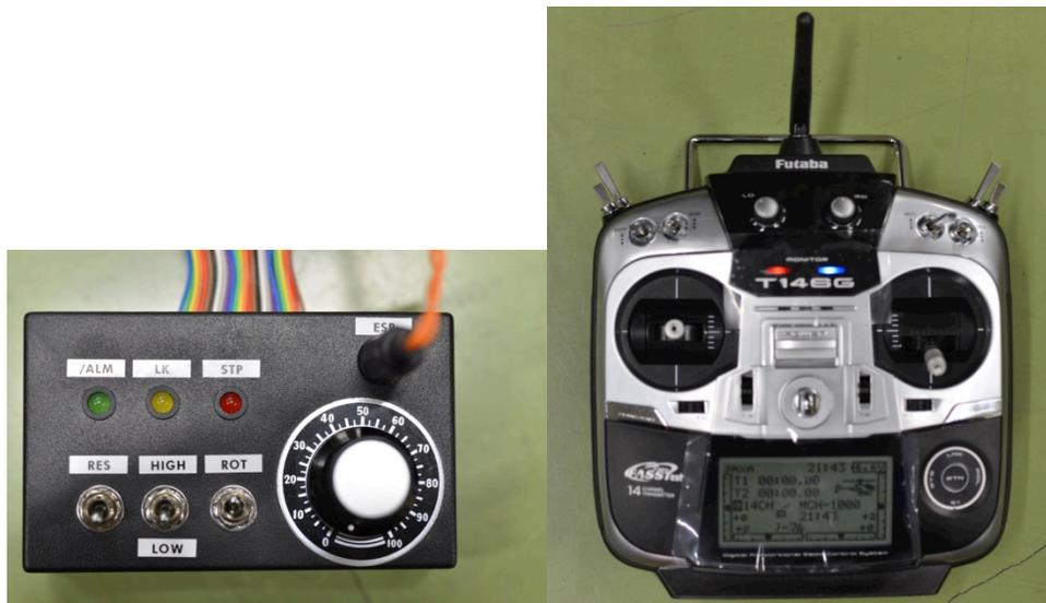
5 Mars controllers. RPM manager (left) all movement remote (right)
