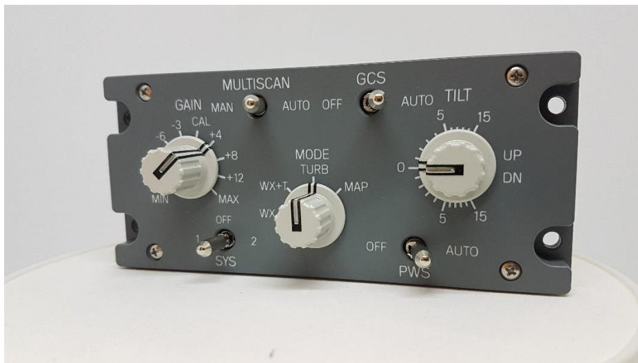
Figura 5.15 – Weather radar panel
