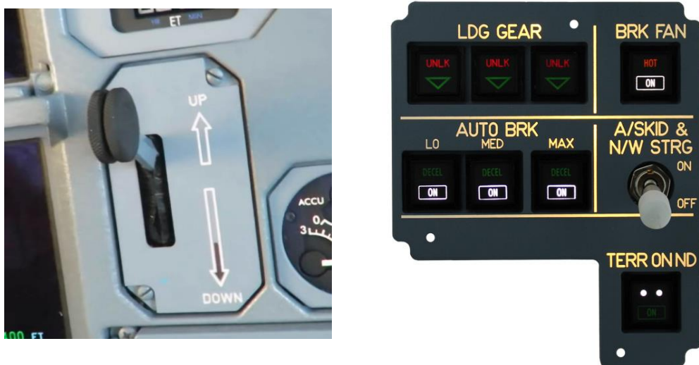
Figura 5.8 – Landing gear lever (sinistra) e landing gear and brakes panel (destra)
