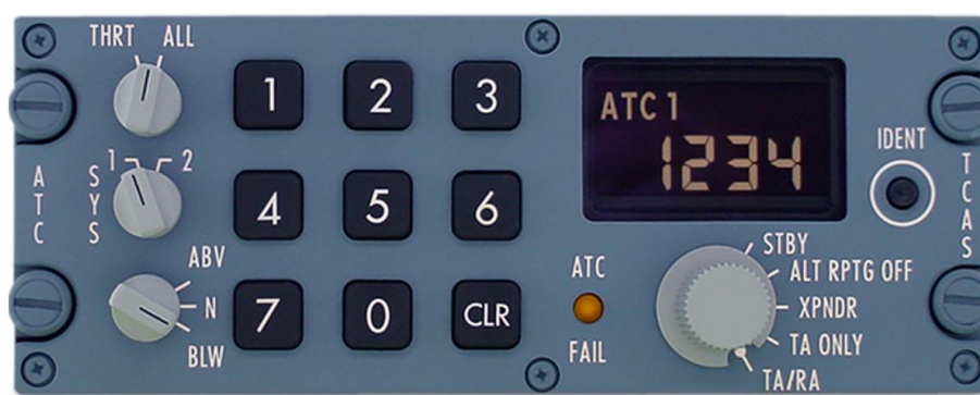
Figura 5.16 – TCAS/ATC Transponder Control Panel
