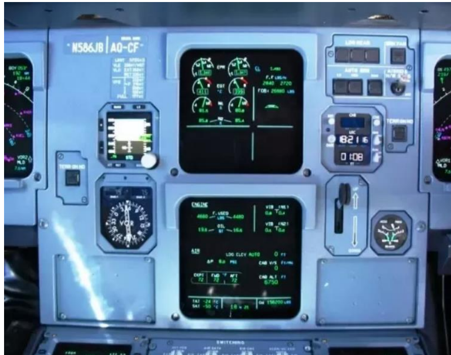
Figura 5.6 – Display dell'Electronic Centralized Aircraft Monitoring
