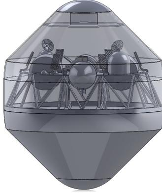
Figure 3.11: CAD Model of the spacecraft encapsulated inside the aeroshell
