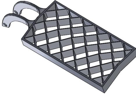
Figure 4.6: Single Grid Fin CAD Model
