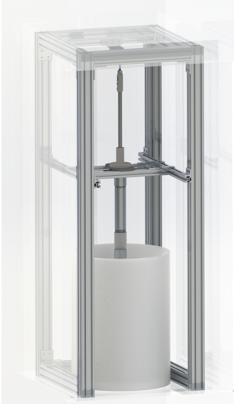
Figure 5.33: Thermal probe / plasma drill experimental setup complete render. The freezer is set as a transparent component.
