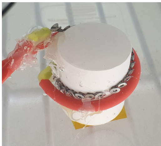
Figure 5.20: Lower inductance, three-gap discharge.
