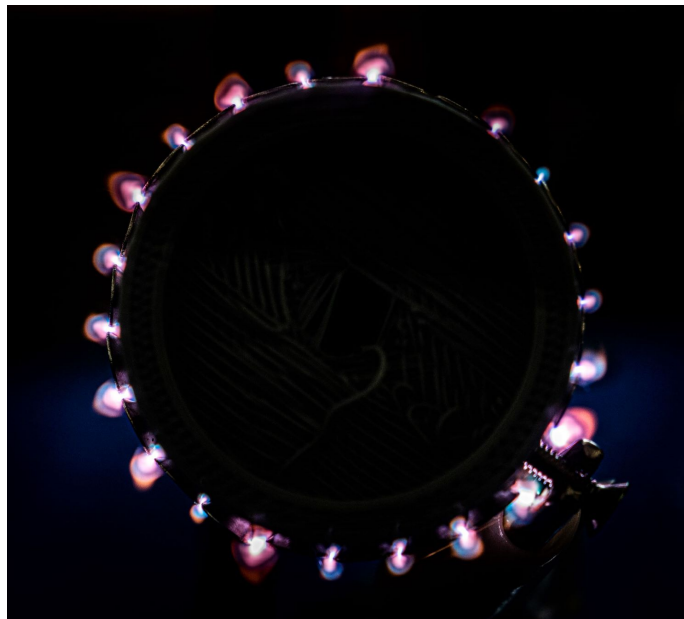
Figure 5.17: Full helical discharge - equally spaced electrodes
