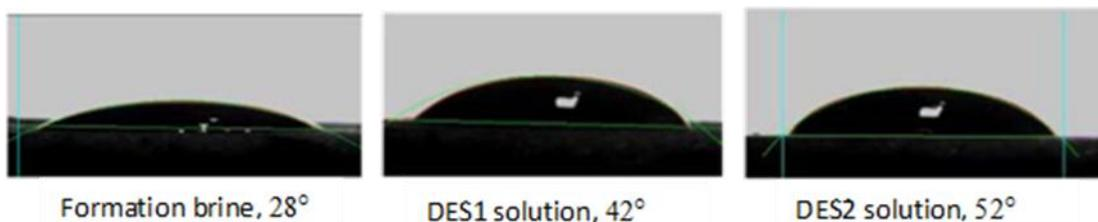
**Fig. 5. 10: Contact angle Measurements with Brine and DES Solutions (Source: Mohsenzadeh et al., 2014)**
