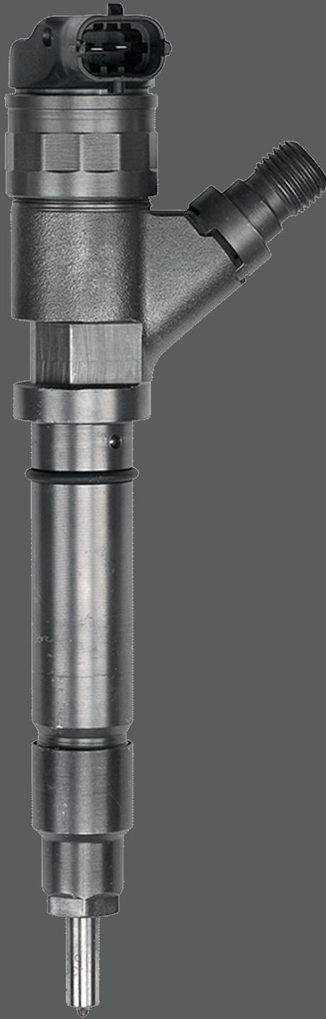
Figure I.45 - CR Solenoid Injector
