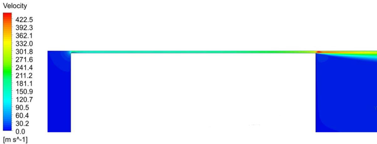
**FIGURE 3.11 VELOCITY BEFORE AND AFTER THE NOZZLE**
