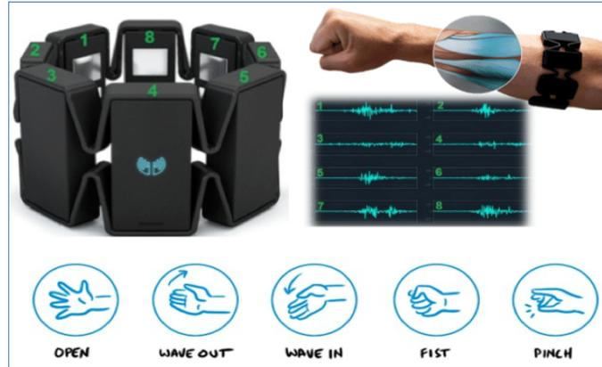
**Figure 2.1:** The Myo gesture control armband. [27]
