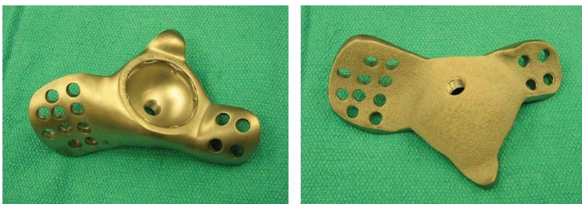
Figure 1.14 – Custom made triflanged acetabular cup from the front (left) and from back (right) view. The backside has a porous coating for long-term biologic fixation. 57
