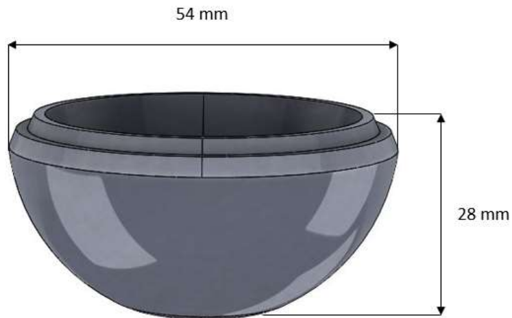
Figure 2.9 - CAD reconstruction of the SeleXys PC ® acetabular cup. The outer diameter and the height of the cup are shown in the figure.
