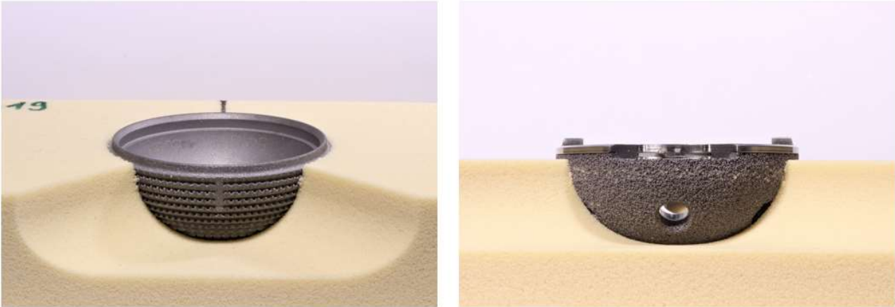
Figure A.1 - Allofit® and TM™ cups after the insertion in the PU-foam block. Allofit® shell in the 90/45 defect block on the left and TM™ shell in the 120/45 defect on the right.
