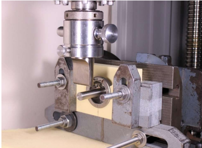
Figure 2.5 - Lever-out test set up. Lever-out test conducted for the TM cup in the PU foam block with the 120/45 defect.
