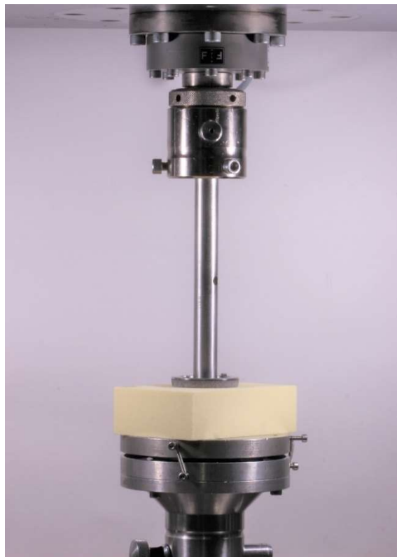
Figure 2.3 – Press-fit test setup. Insertion of the TM cup in the block with the intact cavity. From the upper part of the figure: loading cell, connection adaptor, shaft, cup, artificial bone block, and shear force bearing.
