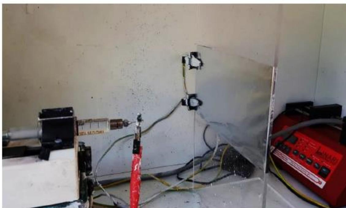
*Fig 35. Electrospinning setup*
