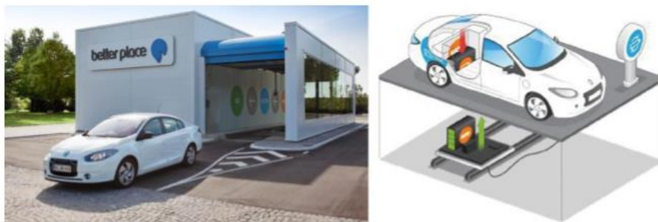
Figure 66. Better place swapping station and operation. Source: [48]
