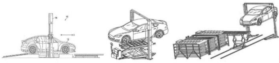
Figure 39. Example of battery swapping operation on a Tesla. Source: [23]
