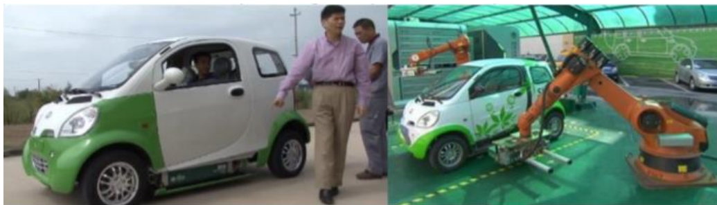
Figure 73. Kandi's Quick Battery Exchange and a mechanical automated arm's operation. Source: [54]
