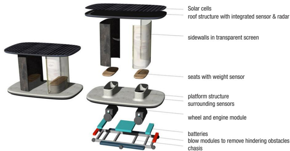
Fig. 2.36. Structural explosion diagram of auto-sliding pavilion
