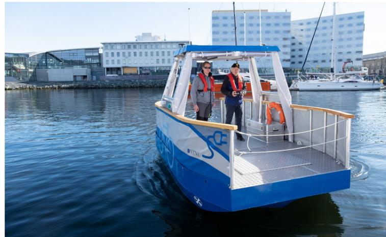
Fig. 2.26. Dragland, K. (n.d.). Autonomous pilot ferry for concept testing and to study behaviour of the other boat traffic. [Photograph]. Retrieved from <https://www.ntnu.edu/autoferry>
