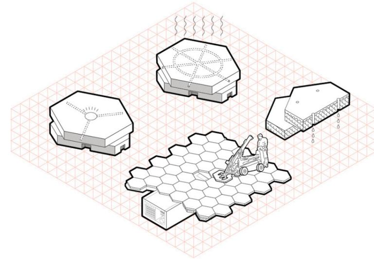
Fig. 2.4. Modularized heated pavement invented by Sidewalk Labs Toronto
