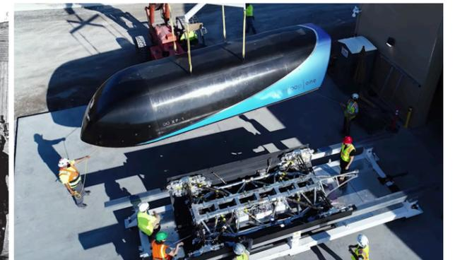
Fig. 2.57. Hosseini, K. (2018). Fuselage and levitating chassis in the process of being seamlessly integrated [Photograph]. Retrieved from <https://hyperloop-one.com/blog/story-radical-hardware>
