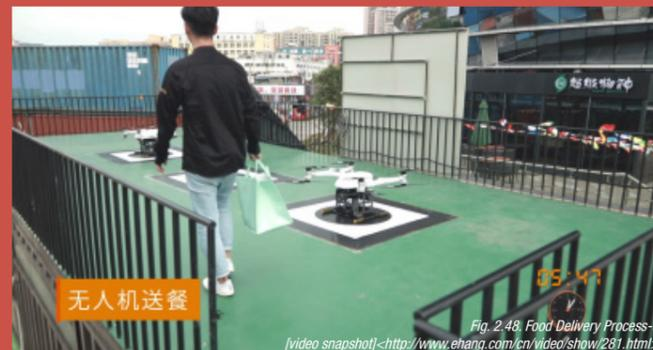
3. Merchants put dishes into the drone and scan the QR code on the aircraft for binding, which is used for customers to check the flight progress on the mobile phone.<sup>1</sup>
