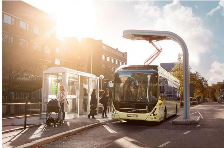
Fig. 2.30. Illustration of a Volvo 7900 electric bus at pantograph charging station in Trondheim
