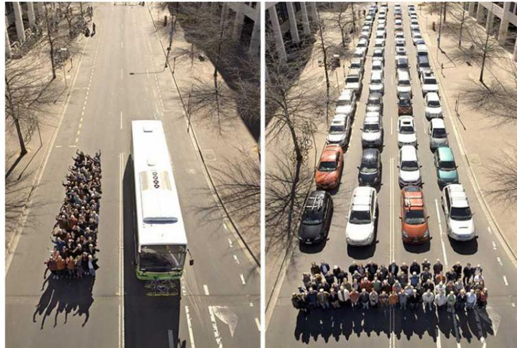
Fig. 2.31. On average, a bus can replace 50 cars. At rush hour, a bus about 16 meters long with a capacity of 74 passengers can stand in line instead of a bus 270 meters long
