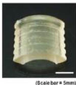
FIGURE 29. CELL-LOADED ARTIFICIAL TRACHEA FABRICATED BY DLP PRINTER (137)
