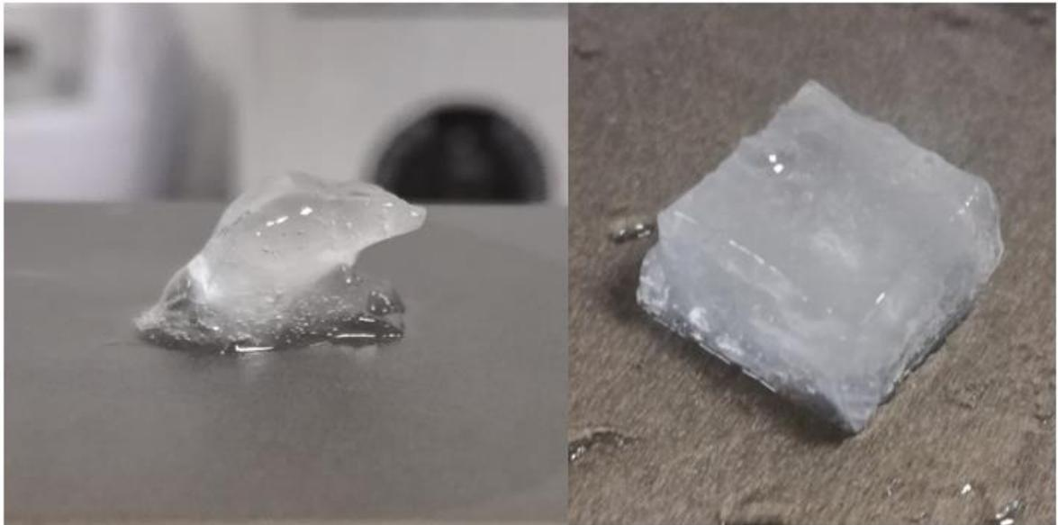
**FIGURE 56. TWO ATTEMPTS TO PRINTING A 30 MG/ML FORMULATION. IN THE SECOND PICTURE, BURN-IN EXPOSURE TIME AND EXPOSURE TIME WERE INCREASED**
