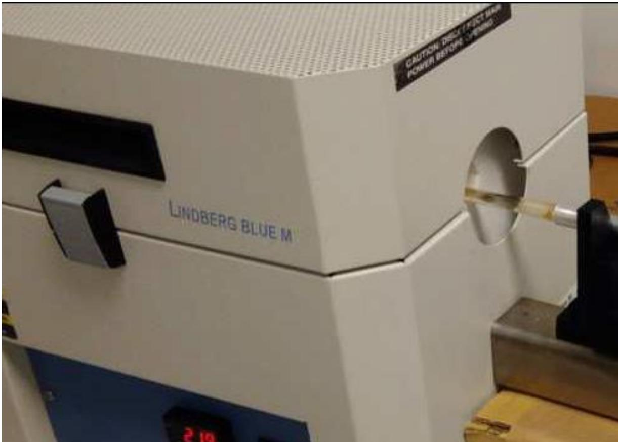
**Fig. 4.12** *Thermo scientific Lindberg/Blue M tube furnace.*
