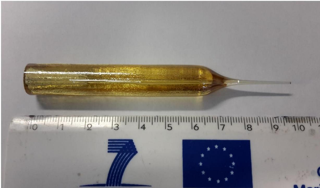
**Fig. 4.8** *Tellurite glass preform produced at Politecnico di Torino.*
