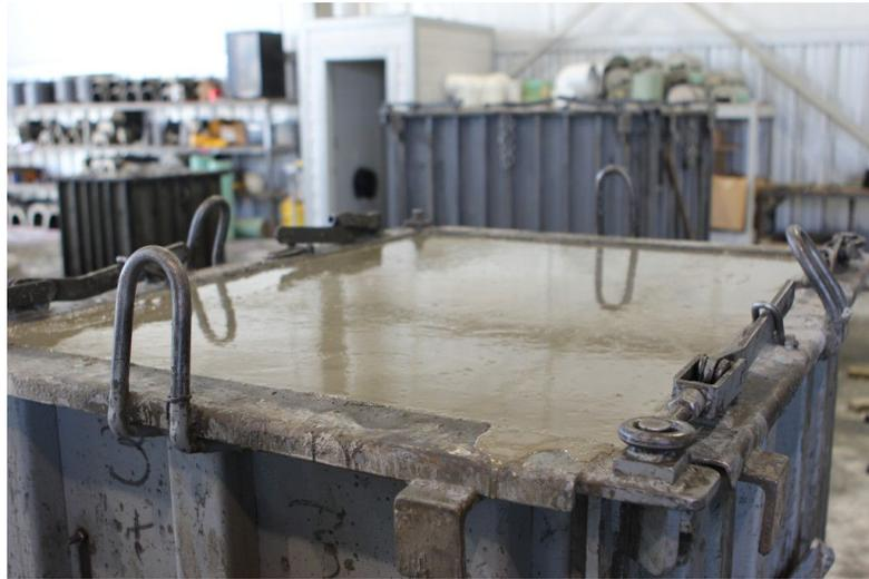
**Figure 3.14:** Picture representing the effect of bleeding.
